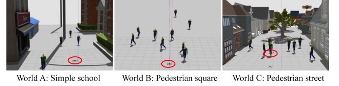
Fig. 7. Simulation worlds. World A: a simple school with very sparse static obstacles, and pedestrians walking slowly (0.5 m/s) in the same direction. World B: a square with dense pedestrians walking in different directions. World C: a street with oak trees and buildings in addition to pedestrians. The walking speed in World B and C ranges from 0.8 m/s to 1.5 m/s.
