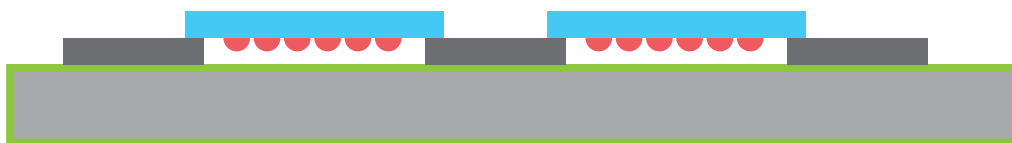
Figure 2.1: Schematic of the gelation chamber. The glass slide is shown in grey, the silicon coating in green, the scotch tape spacer in dark grey, the glass slide in light blue and the cells in red.
