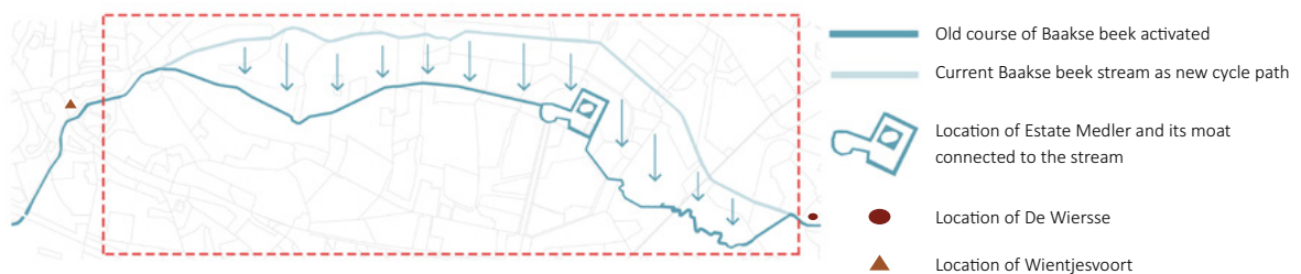
Fig. 7.2 Replacing the existing straightened stream with old meandering stream
