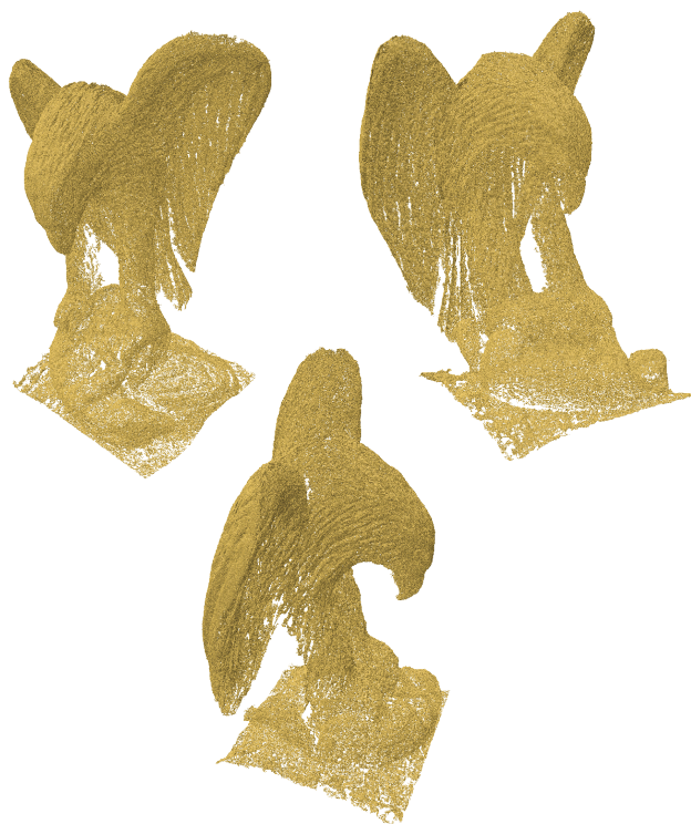
Figure 3. Different views of an eagle point cloud (from Open3D's datasets [18]). The point cloud (796,825 points) contains intricate features, making it an excellent candidate for evaluating reconstruction algorithms.
