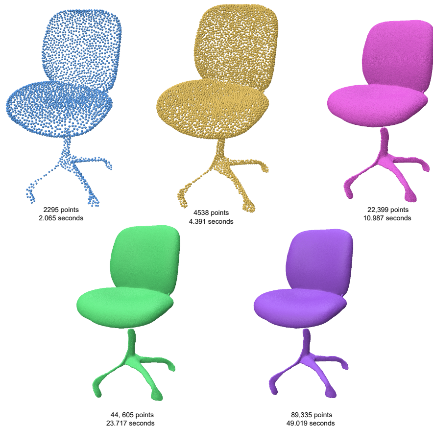
Figure 18. Chair resampled at various sizes using SOLT, along with corresponding sampling times. The results demonstrate that SOLT maintains consistent efficiency and high-quality output as the sample size increases.
