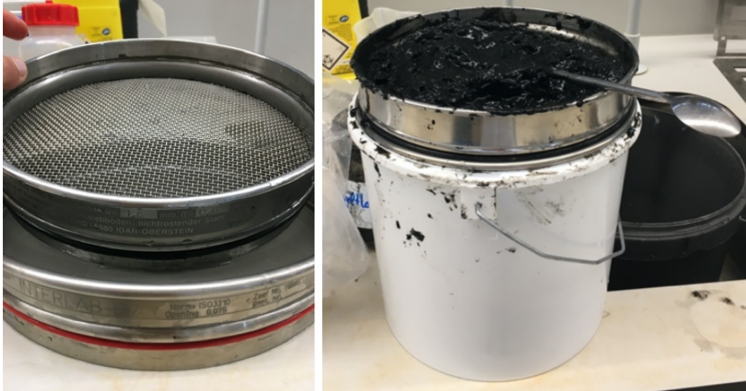
Figure D-5 left: sieves 0.075 and 1.8 mm; right: pre-treatment of the samples by sieving.
