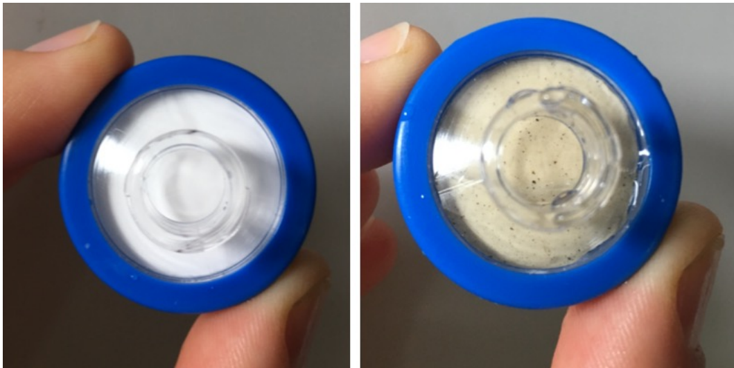
Figure F-4 left: filter membrane before filtration; right: filter membrane after filtration.
