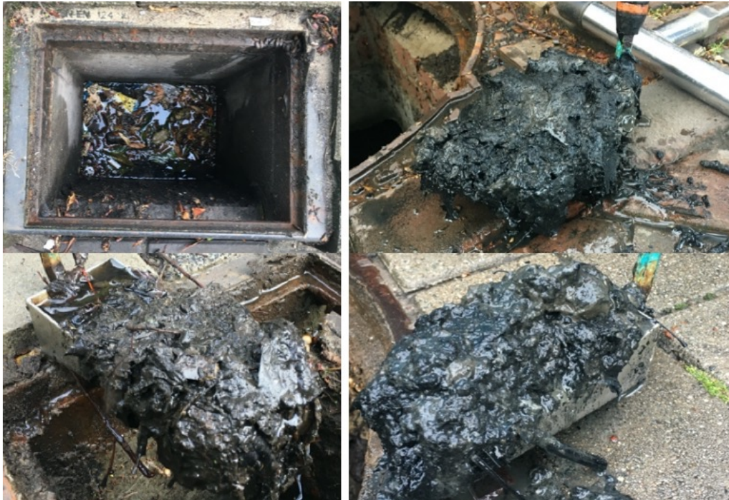
Figure F-1 left: sludge sample from the gully pots; right: sludge sample from the manholes.
