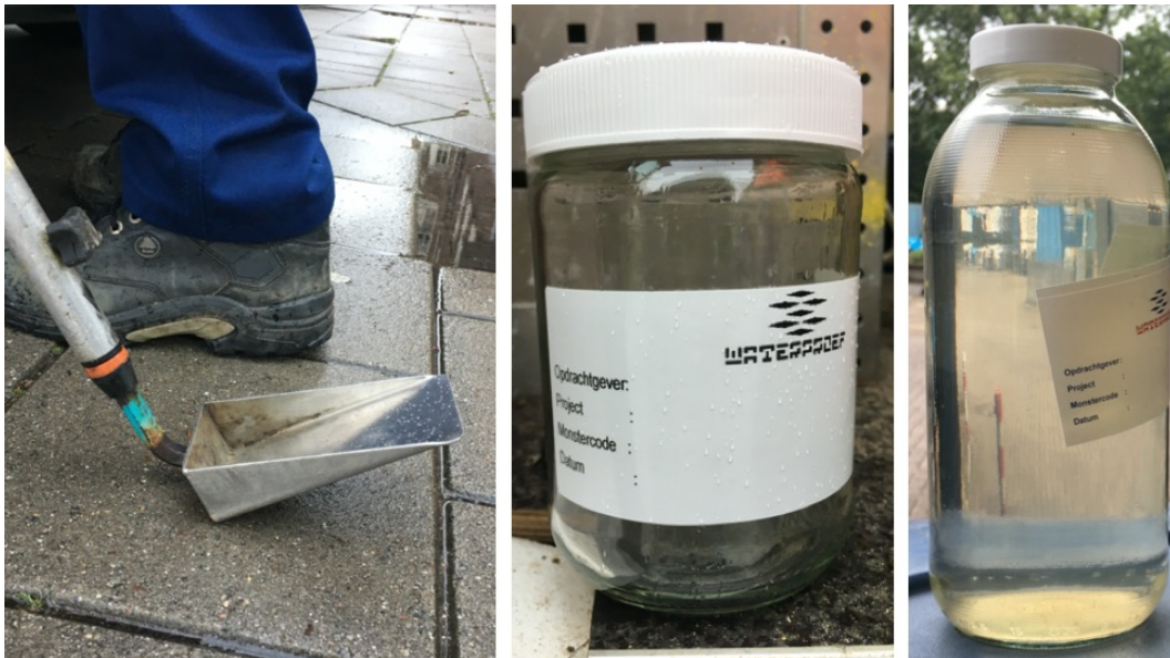
Figure D-4 left: shovel; middle: sampling bottle (550ml); right: sampling bottle (1l).
