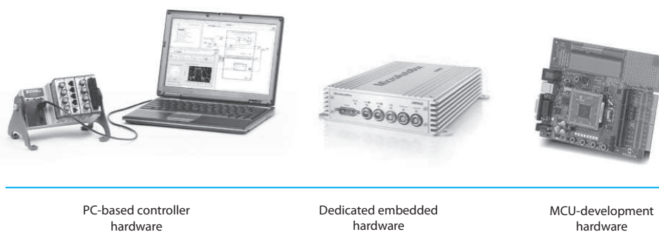
Figure 5-5: A visual comparison between different controller hardware solutions. Each having its own specific strengths and weaknesses in terms of size, weight, I/O connectivity, purchase price and performance.
