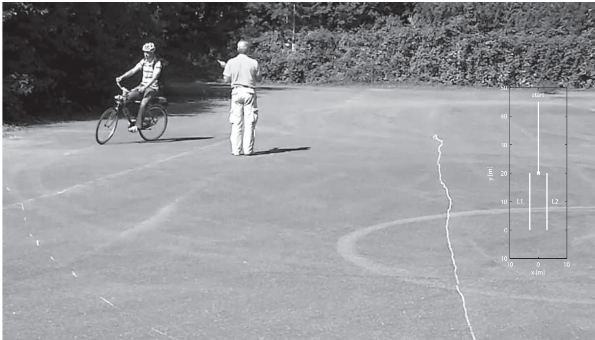
Figure 6-4: Lane change test with the steer-by-wire bicycle at the track along a predefined path as shown on the map overlay. The bicycle is ridden from the start position to halfway of the track at which a sudden left or right direction command is given onto section L1 or section L2.
