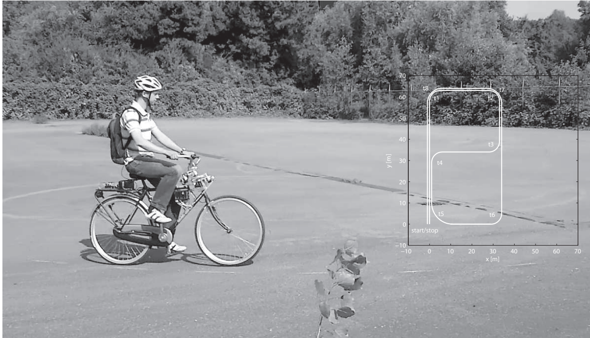
Figure 6-3: Path following test with the steer-by-wire bicycle at the track along a predefined path as shown on the map overlay. A laptop carried in the backpack and connected to the serial-port of the controller was used to store sensor-data and relevant internal controller variables for off-line analysis.
