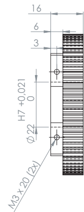
GEAR WHEEL: ANGST + PFISTER 09.1941.1480 TOLERANCES UNLESS OTHERWISE NOTED +0.5 mm
