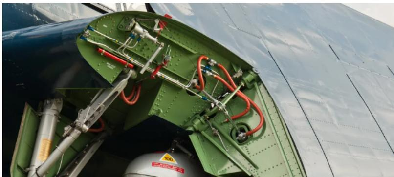
**Figure 14.11:** Grumman F4F-4 Wildcat STO wing folding mechanism
