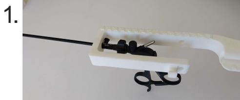
Insert the laparoscopic shaft through the front cavity of the main body.
