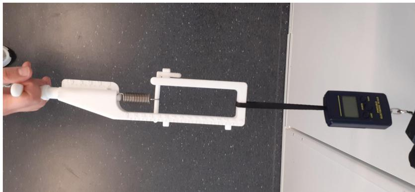
**Figure 8.1:** The setup used for the force measurements. The portable scale (right) is placed in line with the MINT while force is being applied to the handle of the MINT (left).
