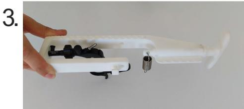
Insert the open side of the spring through the opening in the handle.
