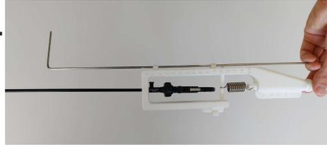
Insert the distance indicator through the holes at the right side of the main body.
