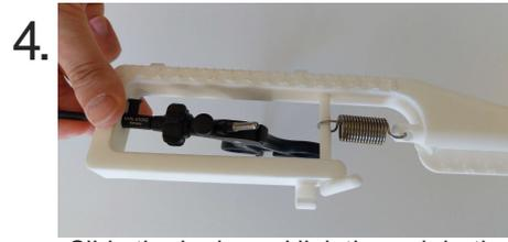
Slide the L-shaped link through both holes in the main body, passing through the closed side of the spring.
