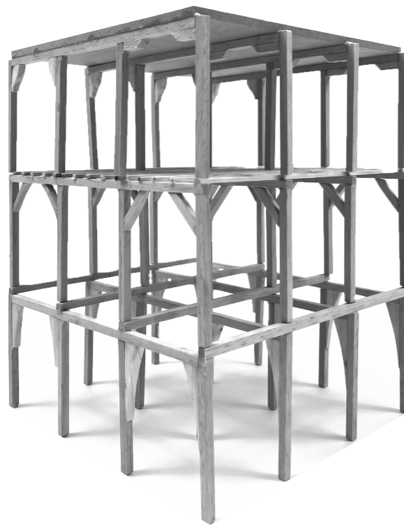
fig. 72: Model exploration of different structural principles based on the Dutch timber tradition
