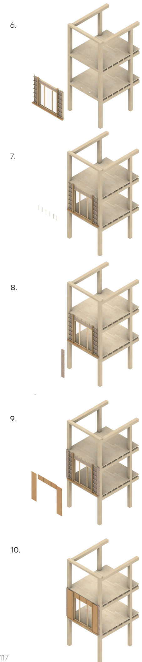
fig. 95: assembly on site of the facade element
