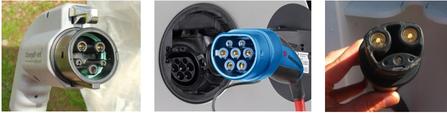
Fig. 2.1. Plug for AC charging- US Type 1 SAE (left), European Type 2 Mennekes (middle) and Tesla plug (right). Image courtesy: Mennekes, Michael Hicks on Wikipedia, insideevs.com
