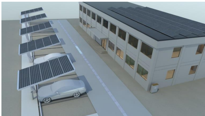
Fig.1.2. An impression of a solar powered EV charging station at workplace where the EVs are charged from PV installed on rooftop and as solar carport (By M. Leendertse)
