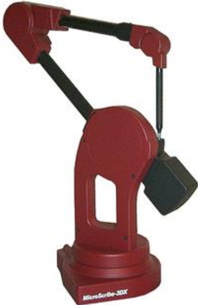
Figure 5. 3D digitizer arm used in [10]
