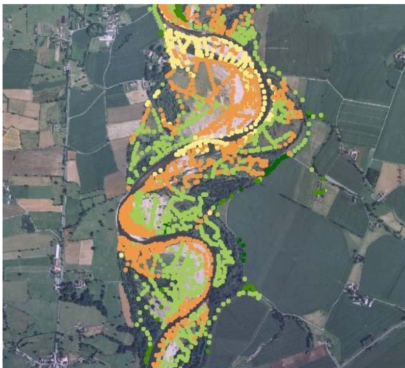
Figure 4–1: Coordinates measured by DGPS in study area. Depicted are the z -values (depth), in French coordinate system Lambert2 ( z=0 reference level is the water level in the harbour of Marseille).
