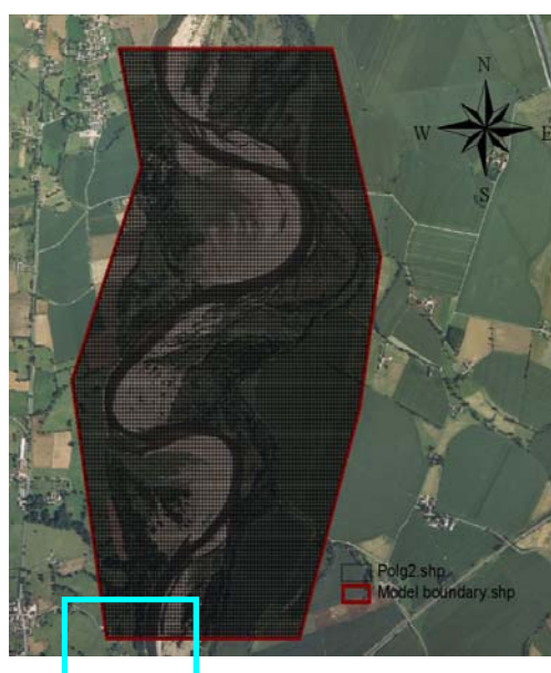
Figure 5-4: Grid of model area with constant gridcell size of 10 x 10 metre.
