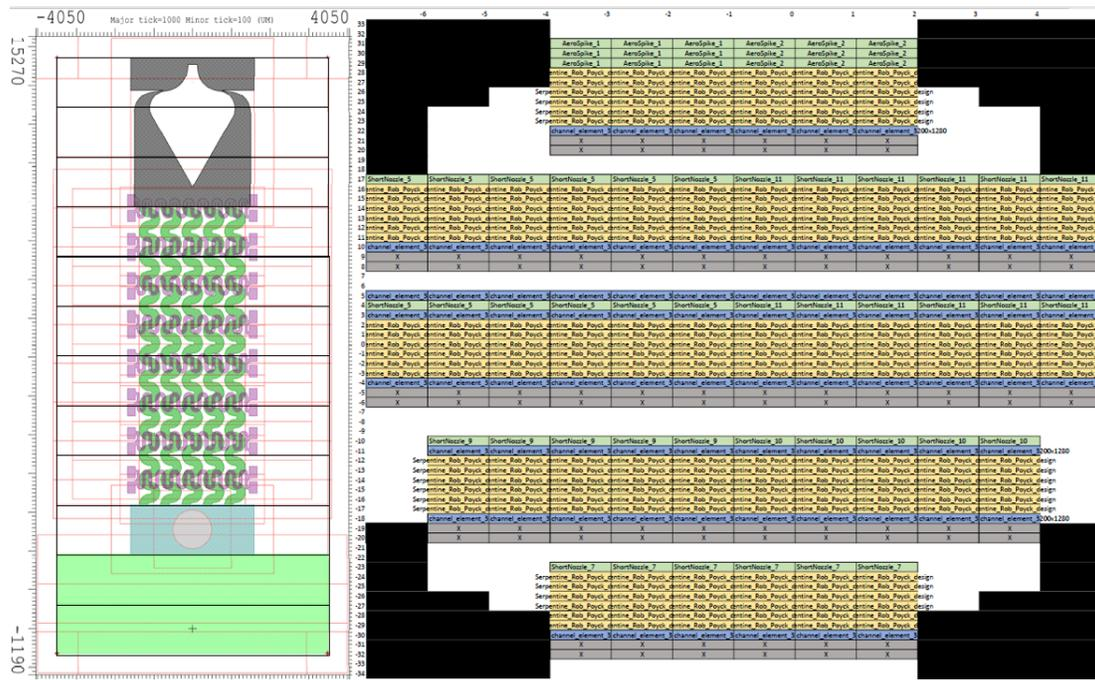
Fig. 5: Wafer configuration : left - an example of modular layout of thruster images in cells(black) ; right - distribution of thrusters across wafer (green signifies nozzle image, yellow is channel and blue is blank image for inlet or spacing, grey implies no image)
