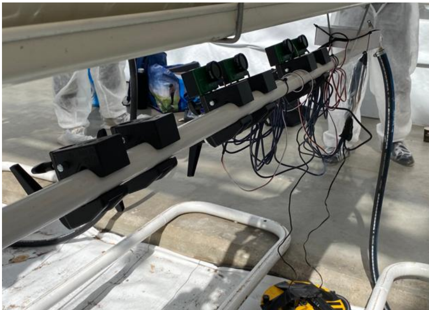
Figure A2: Camera installation for data collection. The cameras were fixed to the heating pipe and connected to the electrical grid with the yellow USB hub.
