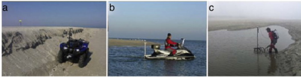
Figure 4.2: The various measuring techniques applied at the Sand Engine; a) ATV next to a beach scarp of approximately 1.3 meter, b) jetski, c) GPS dolly for the lagune. Source: de Schipper et al. (2016).
