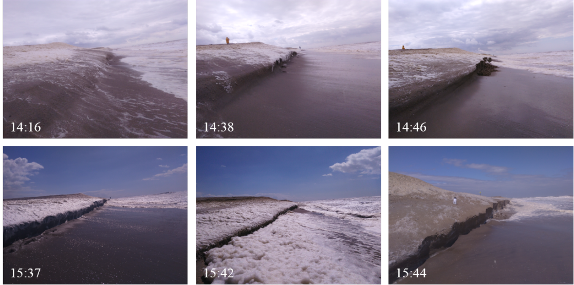
Figure 3.1: Field photographs showing the formation of a beach scarp during summer storm conditions at the Sand Engine (52°03'24.1"N, 4°11'14.6"E). Photo's facing south, taken on 07/06/2017 14:16-15:44 with a water bottle (0.20 m) for scale.
