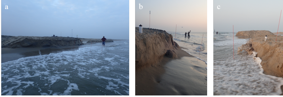
Figure 6.12: Photographs taken of beach scarps at artificial mounts B2 and B3. a) Overview of the two scarps of mount B2 and B3 (left and right within image) on 26/09/2017 08:05. b) Detailed side-view of the beach scarp present at mount B2 on 26/09/2017 19:05. c) Swash impact and reflection on mount B3 on 26/09/2017 19:10. Water bottle (0.2 m) as reference.
