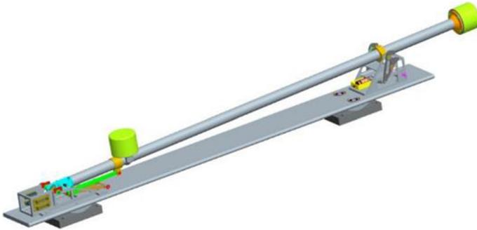
**Fig. 8** Example of developed and tested boom with two flux-gate magnetometers for the KOMPSAT mission
