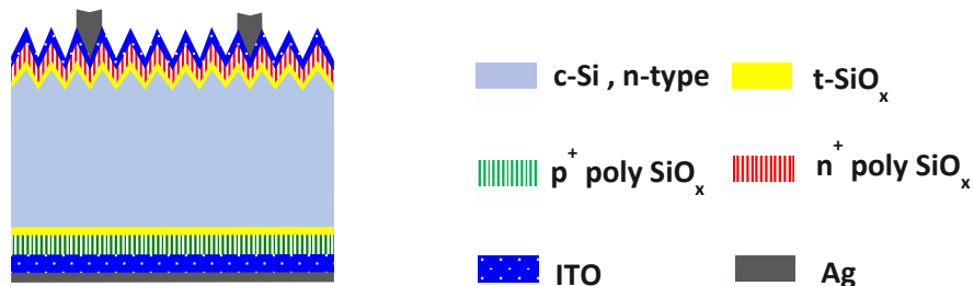
Figure 29 : Schematic structure of FBC solar cell with double ITO layer
