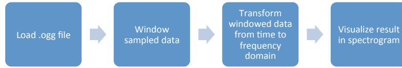
Figure 6.1: Flowchart representing the conversion of raw acoustic data to a spectrogram
