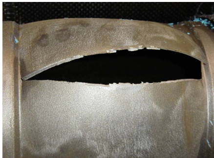
Figure 2.4: Example of a ruptured vessel with an axisymmetric defect [3]
