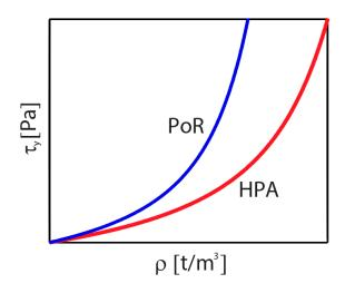
Figure 9: Non-linear relationship between the yield stress  $\tau_{\nu}$  and the density  $\rho$  of mud
