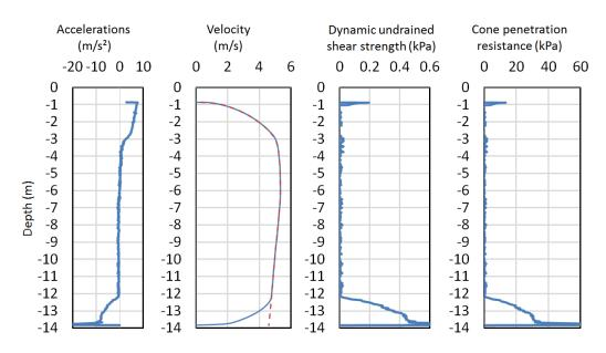
Figure 5: The date measured by the Graviprobe. The fluid mud layer is detected at the depth of -12 m
