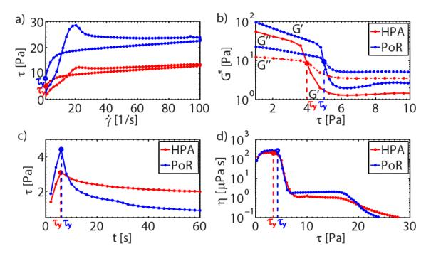
Figure 8: Rheological methods for determining the yield stress  $\tau_y$  of fluid mud at the Port of Rotterdam and the Hamburg Port Authority. a) Thixotropy of mud measured by controlled shear rate experiment. b) Amplitude sweep experiment. c) Stress grow experiment. d) Controlled stress sweep experiment.
