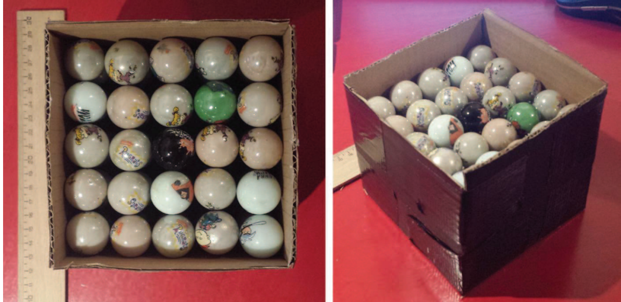
Figure 6-14: Sample of cubic packed uniform spheres.
