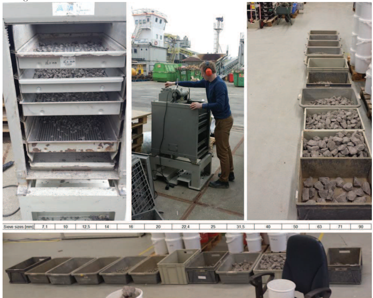
Figure 6-19: Compilation of sieve process.
