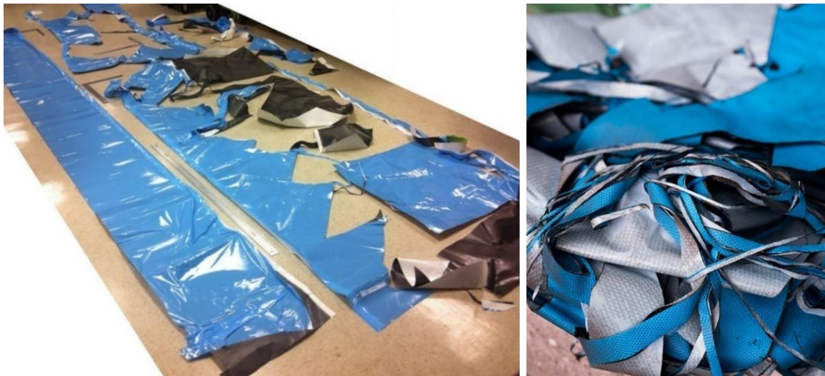
Figure 9 Uncured waste consisting out of prepreg offcut and release film originating from the cutting manufacturing step. Left image [Nilakantan et al. 2015] - Right image [ELG Carbon Fibre Ltd.]
