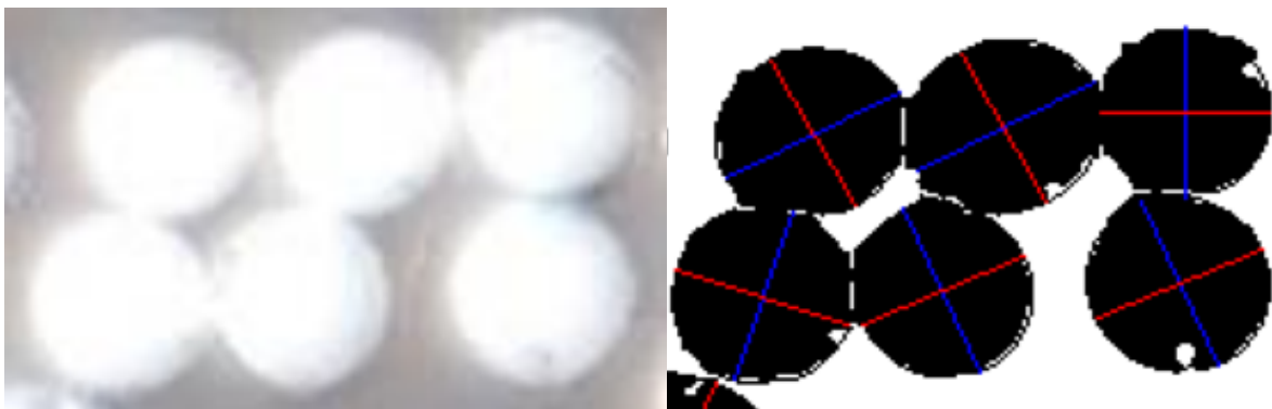
Figure 47 visualisation of minor and major axis measurement on binarized image sample C1 x50
