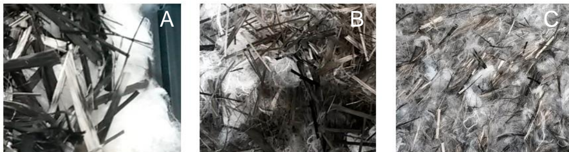
Figure 22 A. CF and PA6 Feedstock. B First & second Opening C mixed feedstock [ J. Wellekötter et al. 2020]
