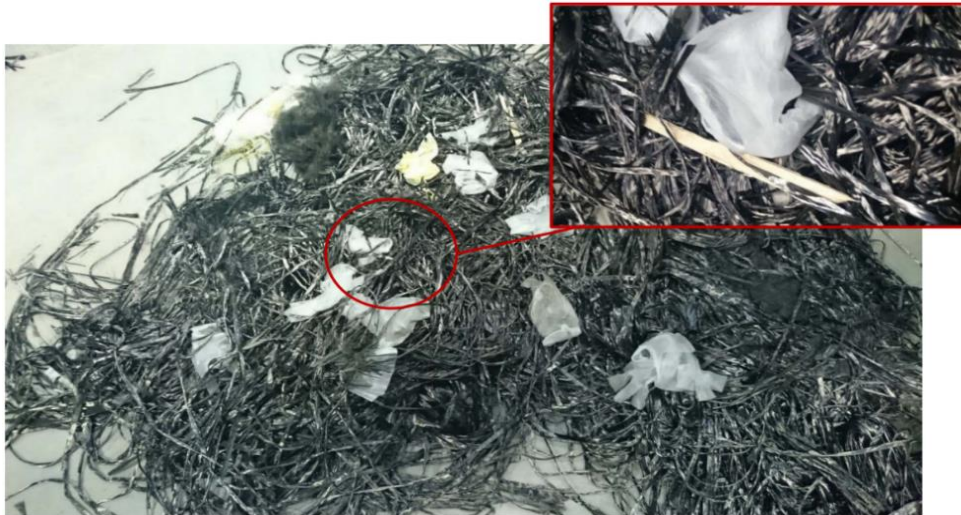
Figure 8 Dry fibre production waste contaminated with various items as received by RecyCarb [Hofmann et al. 2019.]
