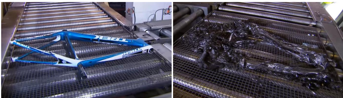
Figure 14 (Left) End of life component before pyrolysis, (Right) End of life component after pyrolysis [CFK Valley Stade Recycling GmbH]
