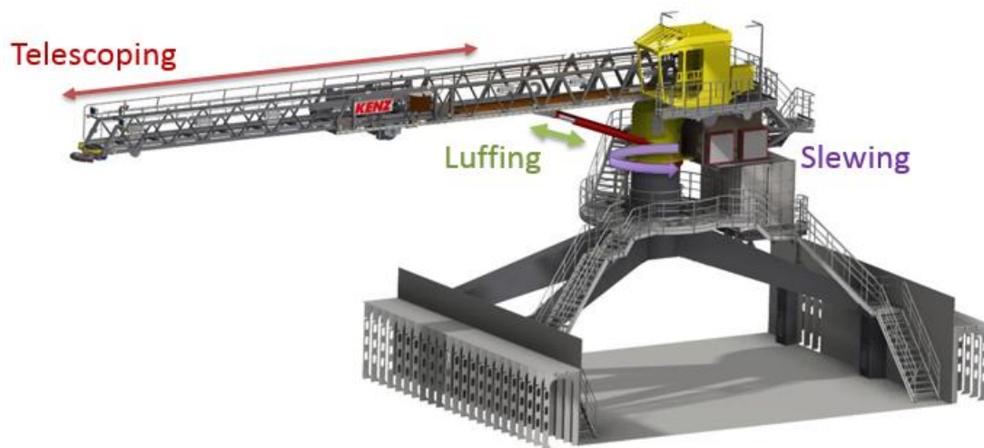
Figure 1.3 - Gangway System with the 3 degrees of freedom indicated
