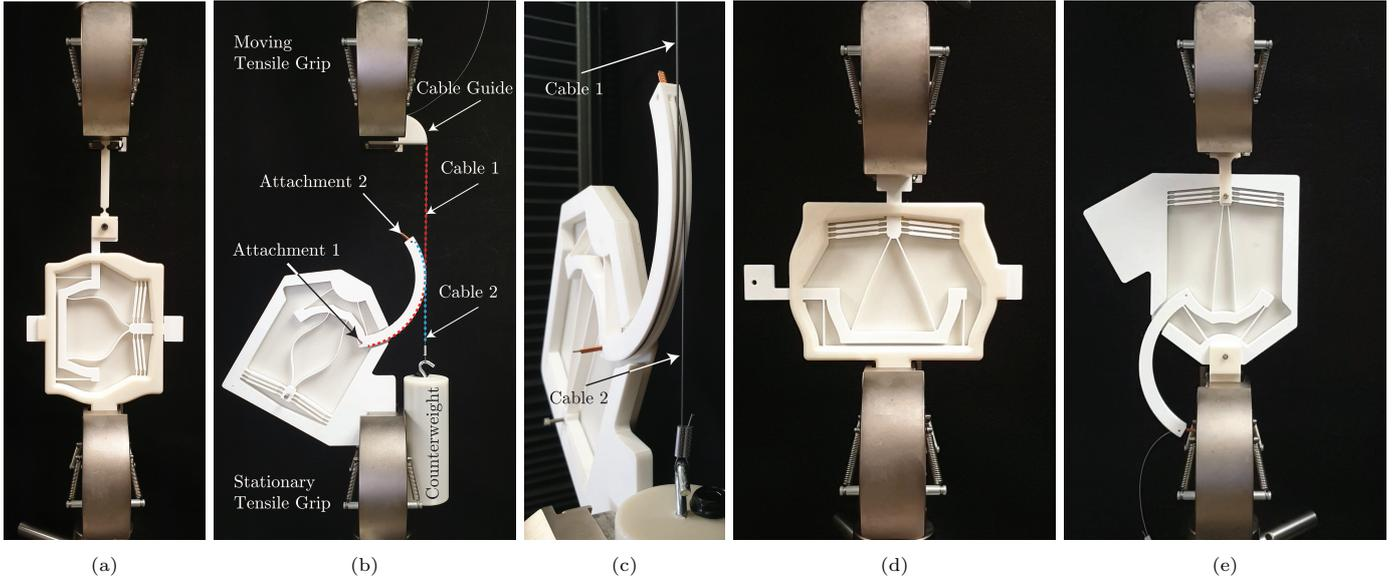
Figure 3: (a) Shows the measurement setup of the linear device. (b) Shows the measurement setup for the rotary device with cable system and preloading weight. (c) Shows how the cables run along grooves in the circular arm of the rotary device. Bistability is measured for the linear device as shown in (d) and for the rotary device as shown in (e).
