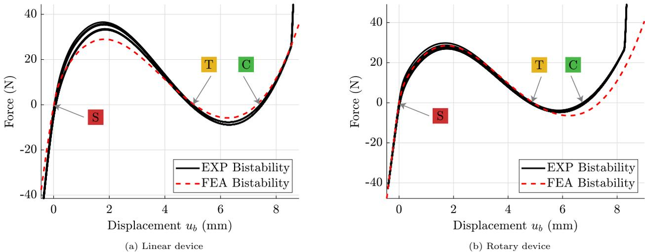
Figure 5: Measurement (EXP) and simulation (FEA) results of the bistable switch are in good agreement for both the linear (a) and rotary (b) device. All equilibrium points are associated with the different states, stiff (S), compliant (C) and toggle (T), as shown in figure 4.
