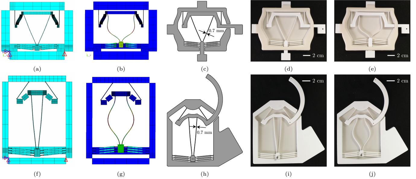
Figure 2: (a, f) Element plots of the linear and rotary devices, (b, g) displacement solutions, (c, h) CAD drawings, (d, i) photos of the prototypes in the stiff state and (e, j) the prototype in the compliant state.
