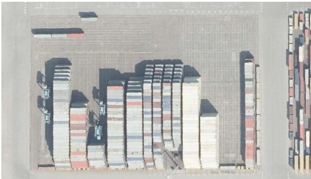
Figure 4.36: Example: empties stack operated by empty handlers (aerial imagery by the National Georegister (NGR) is licenced under CC BY 4.0).
