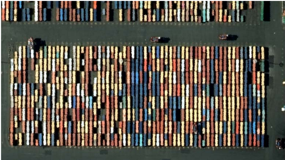
Figure 4.34: Example: ladens stack operated by straddle carriers (aerial imagery by the National Georegister (NGR) is licenced under CC BY 4.0).
