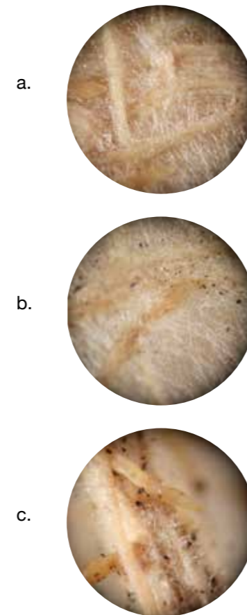
Figure 14. a. Homogeneous, b. heterogeneous and c. patterned sample under microscope (4.5X)
