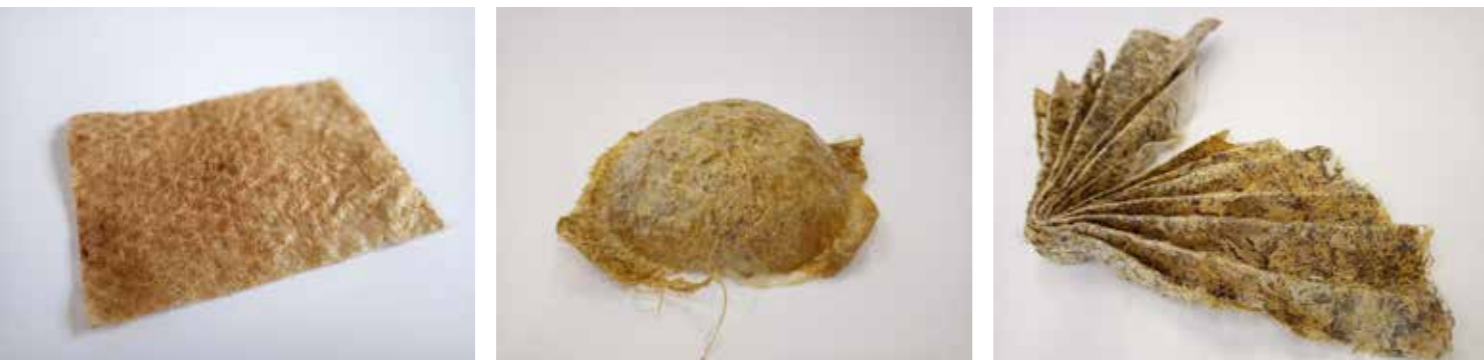
Figure []: Bioplastic bonded to Interwoven samples, exhibiting changes in form during and after curing
