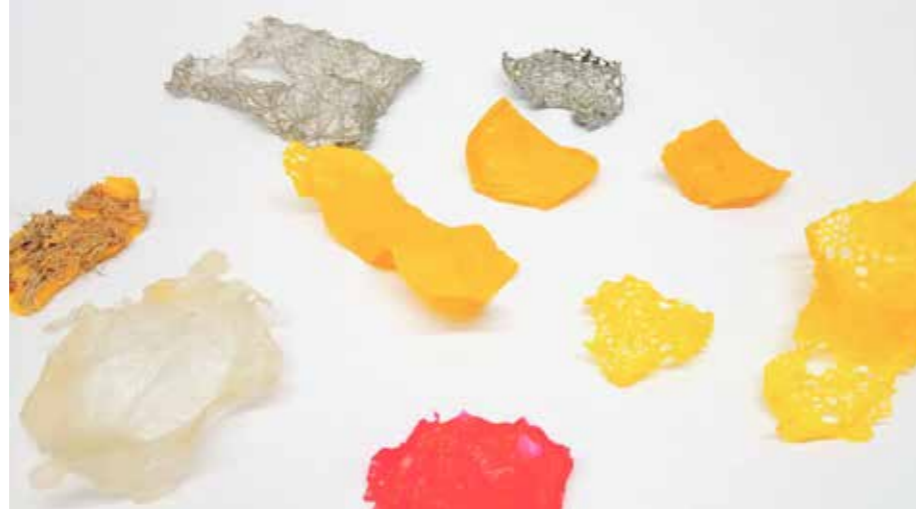
Figure 38 . Initial samples of alginate bioplastic made at Waar Society
