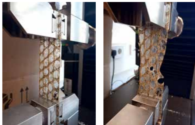
Figure 79: Hexagon samples being tested during and after failure
