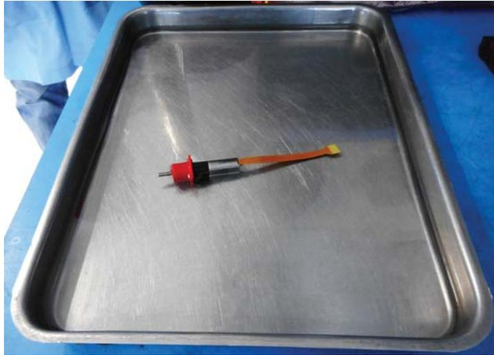
**Figure 3.11:** Maxon motor with planetary gearhead under thermal test
