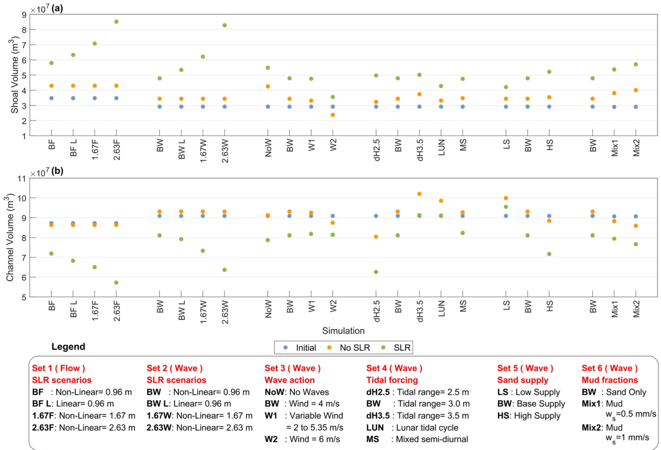
Figure 9. Summary of the sensitivity analysis for different forcing conditions showing (a) the shoal volume ( \text{m}^3 ; w.r.t LW), and (b) the channel volume ( \text{m}^3 ; w.r.t LW) for the whole model domain for the initial state (blue), after 100 years without sea-level rise (SLR) (Orange), and after 100 years with SLR (Green). The legend presents the abbreviations used for the different simulations and the description of the varying forcing condition. BF and BW refer to the Base Flow and Base Wave simulations, respectively.
