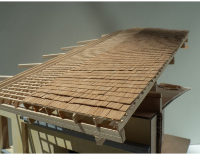
1:20 sectional fragment model, pictured from the roof
