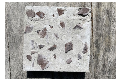
Material sample from re-using brick into cyclopean concrete. Testing different pouring and polishing techniques.
