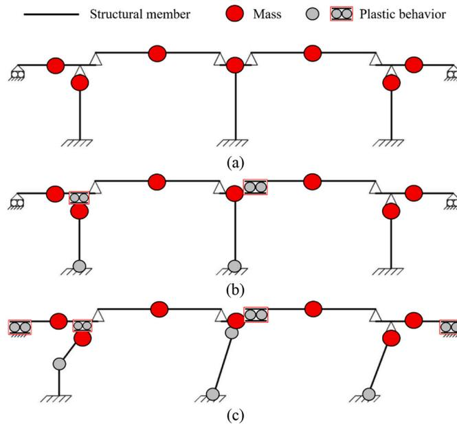
Fig. B4. Possible mechanisms in the longitudinal direction. a) simplified sketch of the bridge; b) a mixed mechanism without corrosion; c) a mixed mechanism with corrosion in columns only.
