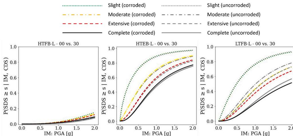
Fig. B5. Fragilities of BEA components in the longitudinal direction. a) HTFB scenario 00 vs. 30; b) HTEB scenario 00 vs. 30; c) LTFB scenario 00 vs. 30.
