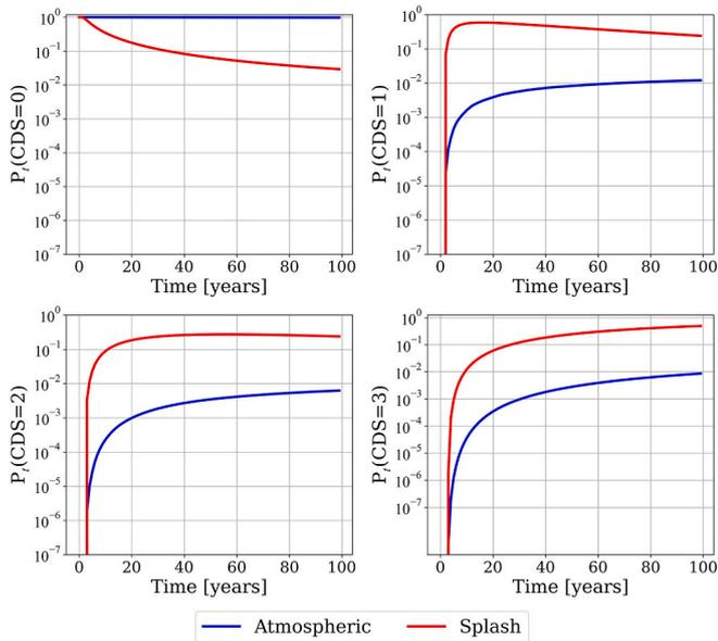
Fig. 14. Probabilities of corrosion deterioration states ( $P_{CDS}$ ) of structural components over their lifetime.
