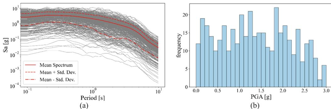
Fig. 6. Characteristics of the ground motion suite. a) Spectral acceleration vs. period; b) peak ground acceleration distribution.
