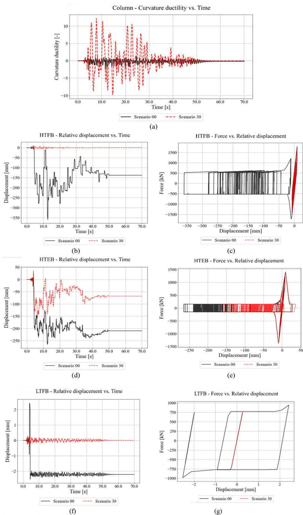
**Fig. B3.** Time history analysis of the EDP for bridge components under the same ground motion. a) COL curvature ductility; b) HTFB relative displacements; c) HTFB force vs. relative displacement; d) HTEB relative displacements; e) HTEB force vs. relative displacement; f) LTFB relative displacements; g) LTFB force vs. relative displacement.
