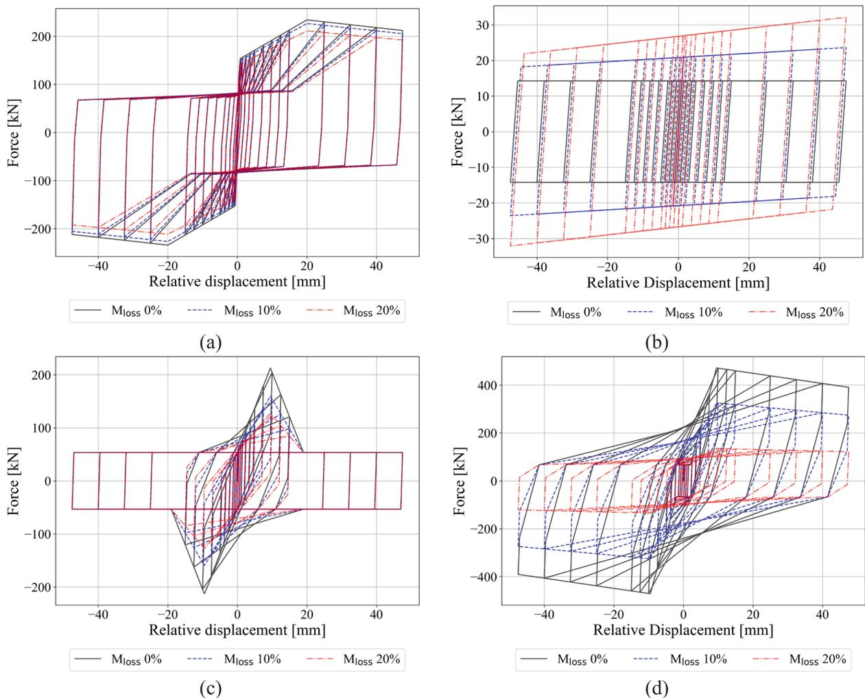
Fig. 10. Cyclic behavior of bearing components under uncorroded and corroded cases.
