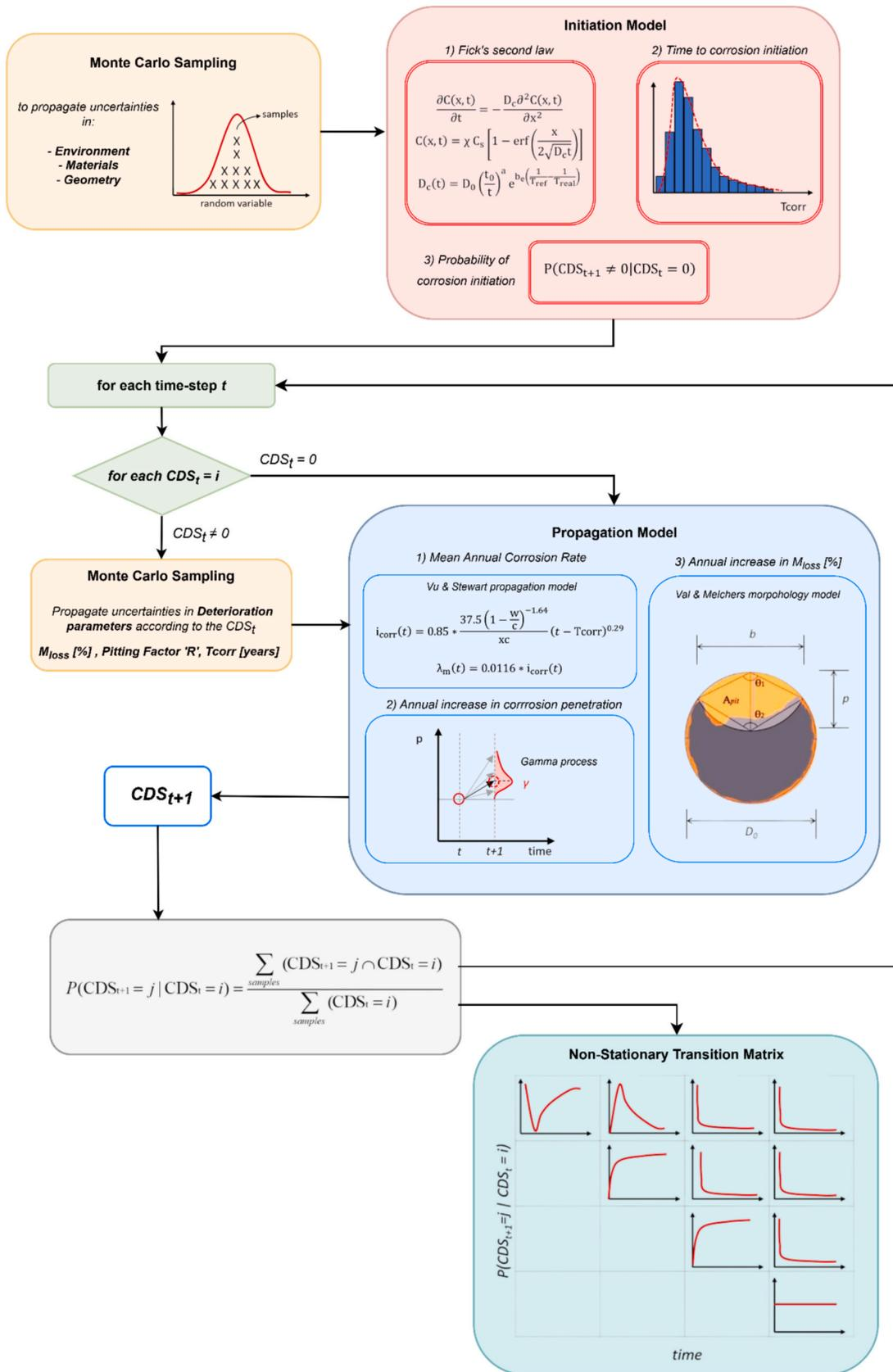
Fig. 3. Flowchart for the proposed methodology to compute the non-stationary transitions.
