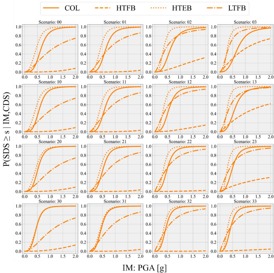
Fig. 16. State-dependent fragilities for the Moderate SDS of the case study bridge components according to 16 scenarios. Scenario  $ij$ :  $i = CDS_{COL}$ ,  $j = CDS_{BEA}$ .
