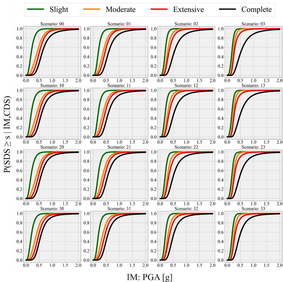
Fig. 19. State-dependent fragilities across the four SDS of the case study system according to 16 scenarios. Scenario  $ij$ :  $i = CDS_{COL}$ ,  $j = CDS_{BEA}$ .
