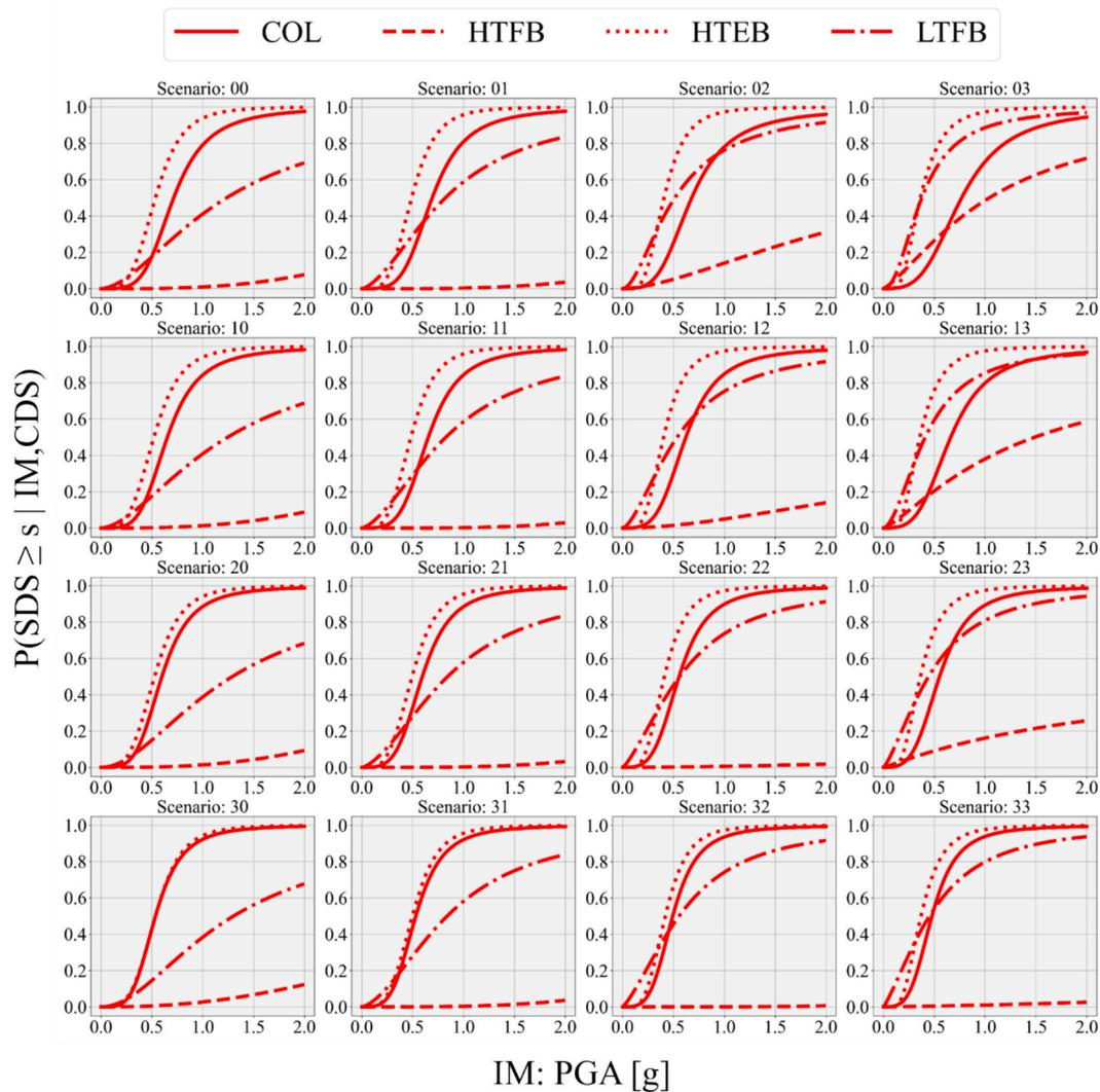
Fig. 17. State-dependent fragilities for the Extensive SDS of the case study bridge components according to 16 scenarios. Scenario  $ij$ :  $i = CDS_{COL}$ ,  $j = CDS_{BEA}$ .
