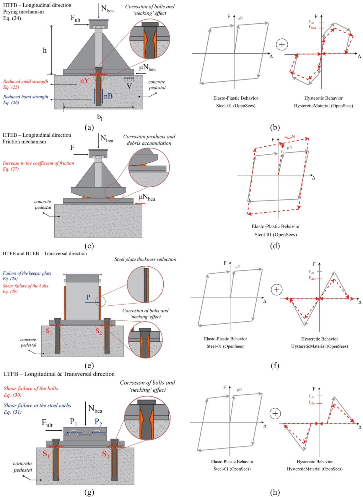
Fig. 9. Corrosion modeling assumptions in bearing components, modified according to [53].
