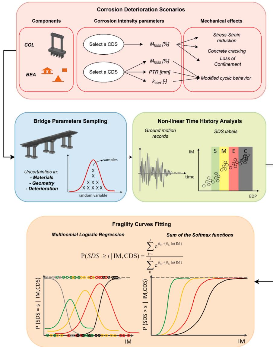
Fig. 5. Flowchart for the methodology to evaluate the state-dependent fragility curves.
