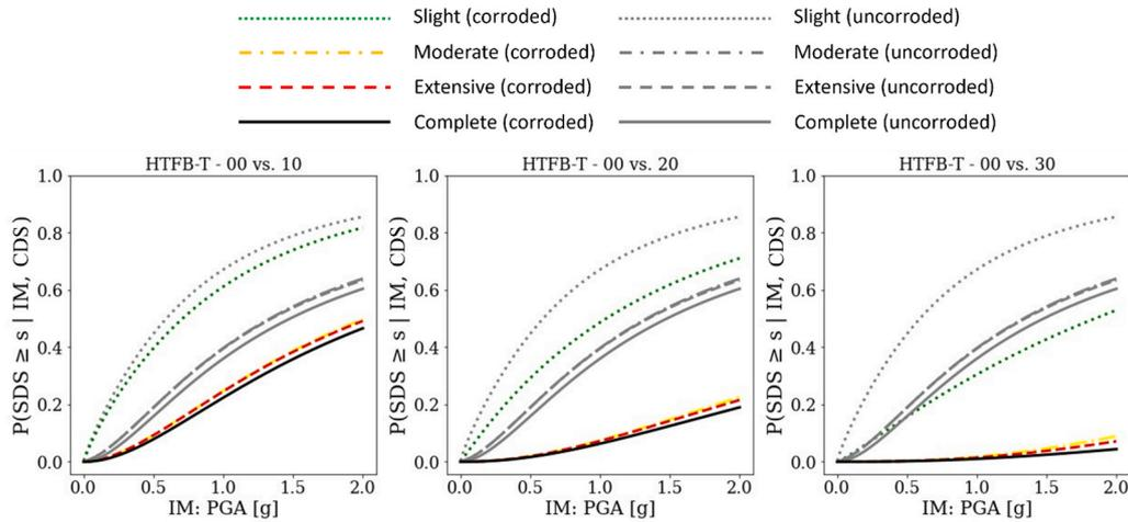
Fig. B1. Fragilities of HTFB in the transverse direction. a) scenario 00 vs. 10; b) scenario 00 vs. 20; c) scenario 00 vs. 30.
