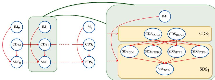
Fig. 2. DBN for life-cycle seismic fragility of deteriorating bridges. The overall model including nodes and transitions (left) and interactions among component and system states within a single time step (right). COL = columns; HTFB = high type fixed bearings; HTEB = high type expansion bearings; LTFB = low type fixed bearings; SYS = system.
