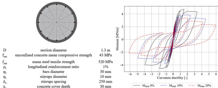
Fig. 8. Cyclic behavior of column components under uncorroded and corroded cases.
