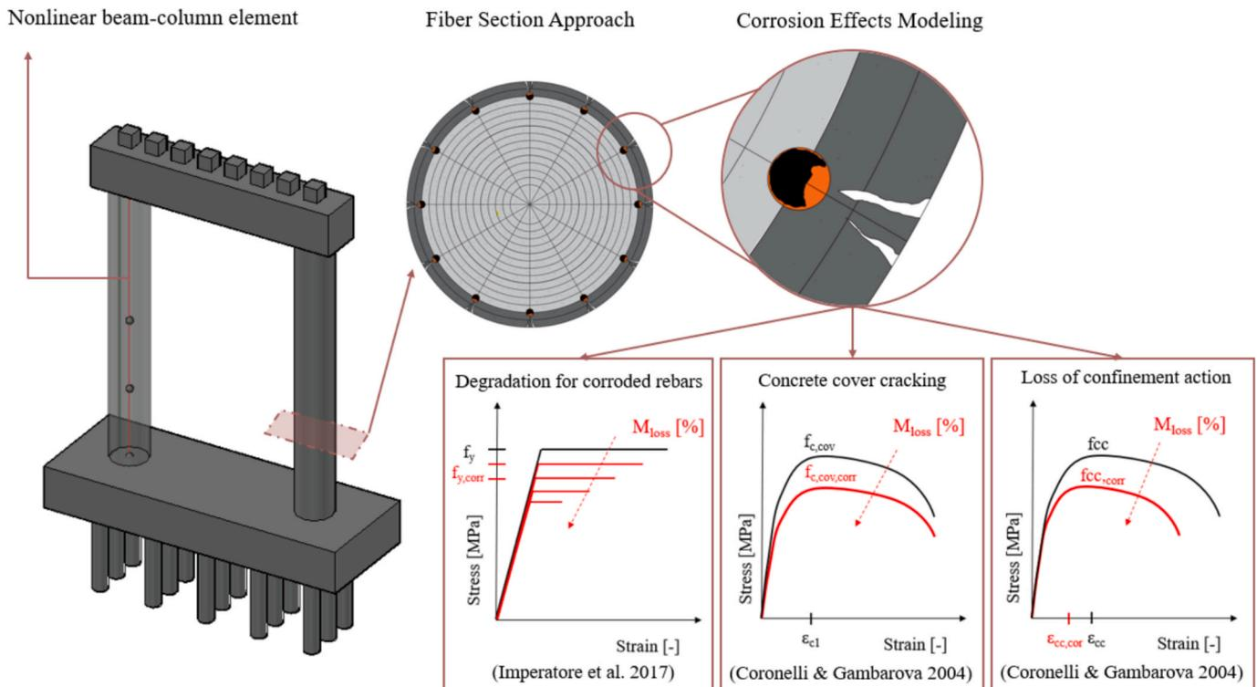
Fig. 7. Corrosion modeling assumptions in column components.
