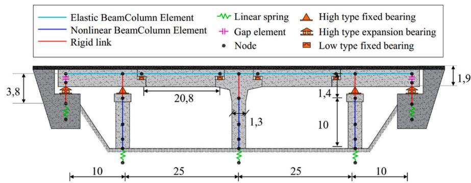
Fig. 11. The 4-span bridge case study with respective geometrical and finite element modeling features. Modified after [36].
