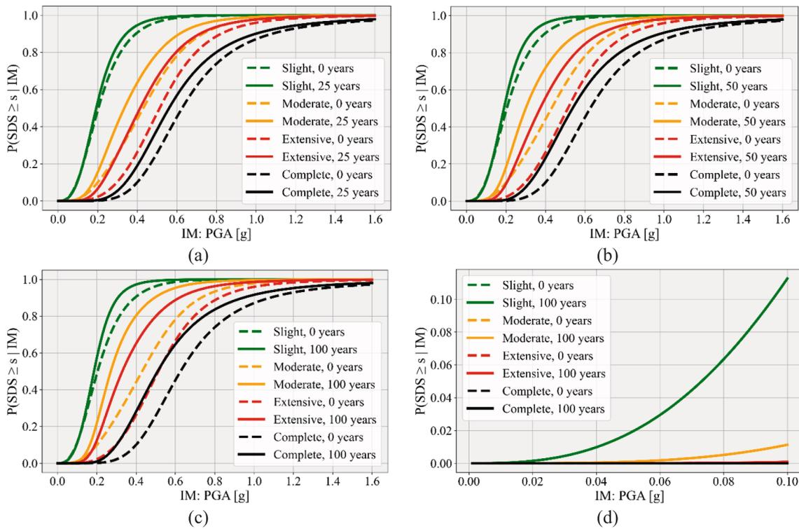
Fig. 20. System fragilities over the life-cycle of the case study bridge under different environmental conditions. a) Splash – 25 years; b) Splash – 50 years; c) Splash – 100 years; d) Atmospheric – 100 years.
