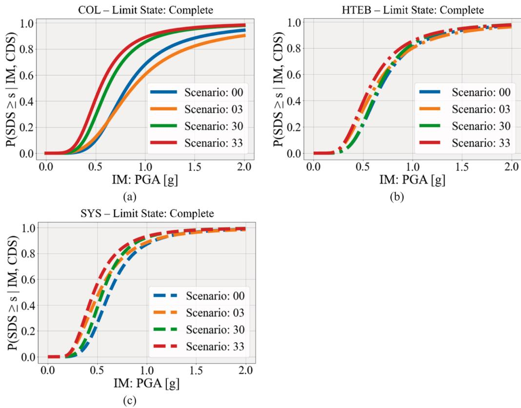
Fig. 21. Effects of specific corrosion scenarios on the seismic fragility of critical components and the system. a) COL components; b) HTEB components; c) System.
