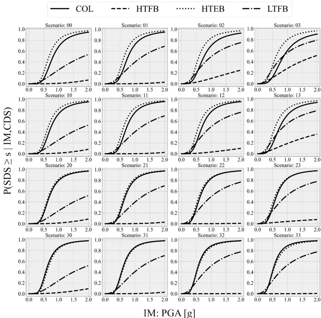
Fig. 18. State-dependent fragilities for the Complete SDS of the case study components according to 16 scenarios. Scenario  $ij$ :  $i = CDS_{COL}$ ,  $j = CDS_{BEA}$ .
