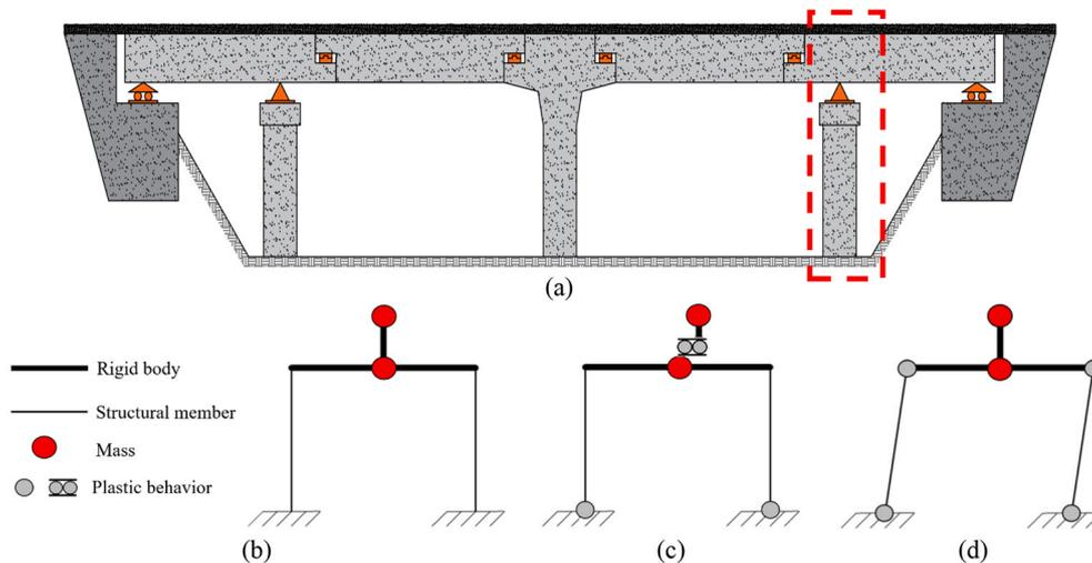
Fig. B2. Possible mechanisms for the COL-HTFB subsystem in the transverse direction. a) sketch of the bridge; b) simplified model of the transversal COL-HTFB subsystem; c) mixed sidesway mechanism; d) column sidesway mechanism.
