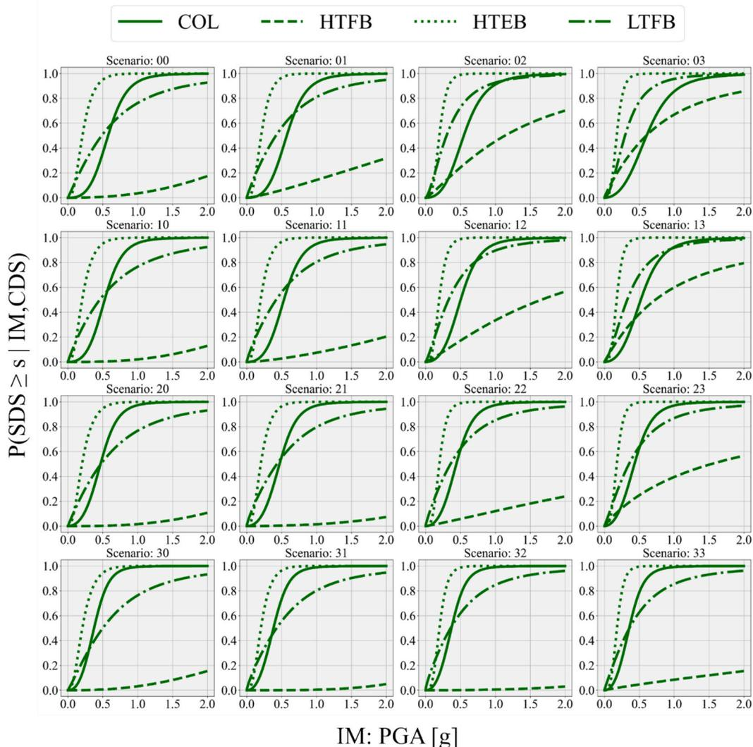
Fig. 15. State-dependent fragilities for the Slight SDS of the case study bridge components according to 16 scenarios. Scenario  $ij$ :  $i = CDS_{COL}$ ,  $j = CDS_{BEA}$ .
