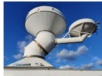
Fig. 2. S- / X-band high-resolution Doppler polarimetric FMCW radar [21].
