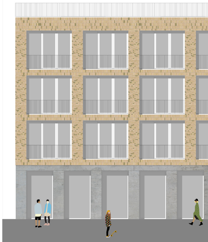
Image 15 Yellow brick with light gray joint tested in facade (own image)
