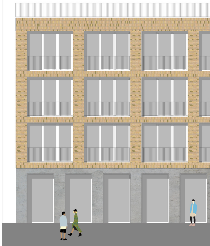
Image 13 Yellow brick with yellow joint tested in facade (own image)
