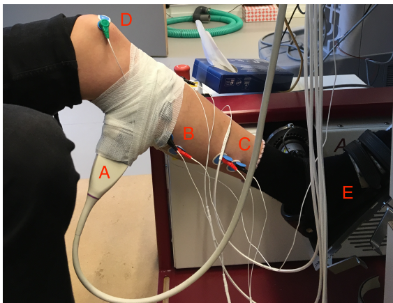
Fig. 3: Experimental set-up which shows the participants foot strapped to the ankle manipulator (E). The ultrasound probe and self-adhesive bandaging can be seen at A. The EMG electrodes attached to the skin are placed above the GM muscle as seen at B and above the SOL muscle as seen at C (Electrodes are also placed on the TA and GL, but not visible here). A ground electrode is placed on the kneecap at D.
