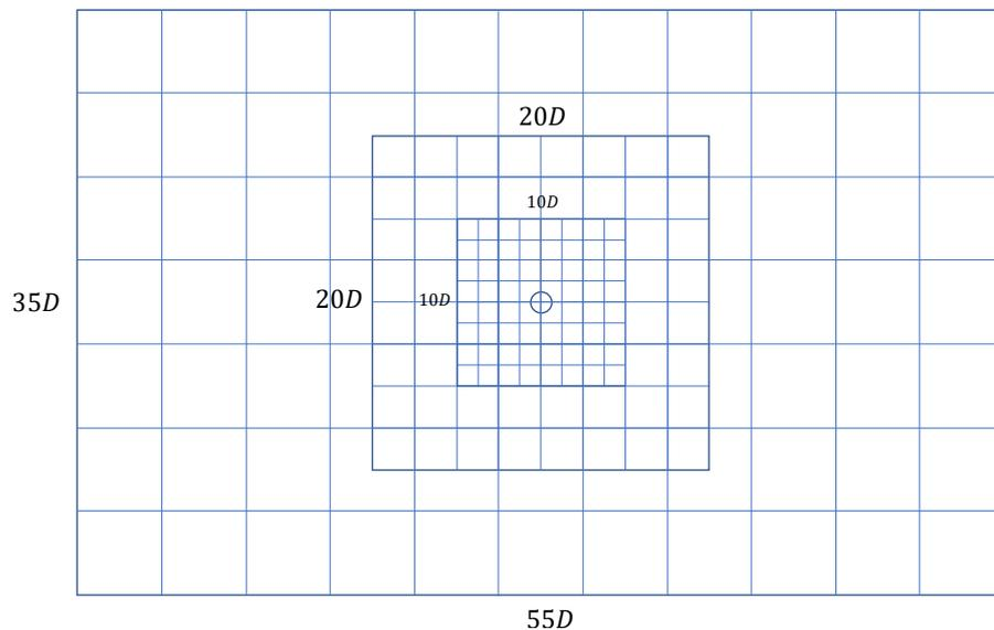
Figure 8.1: Domain and grid discretisation of the flow around and oscillating cylinder in a fluid at rest. A multi-grid is used, with the innermost, finest square having double the grid refinement of its parent grid, which in turn has a twice as fine grid as the background grid that covers the full domain.
