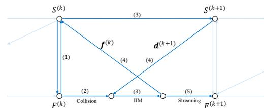
Figure 6.4: Discretisation of a boundary, with fluid nodes (as used by the IBM/IIM by the fluid solver described in Chapter 4 and 5) and structural nodes (as used by the structural model described in Section 6.1).
