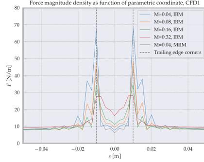
Figure 9.7: Plot of the boundary force distribution at the tip of the flag, for different Mach numbers, for CFD1 at a mesh discretisation such that  $R = 20\Delta x$ .
