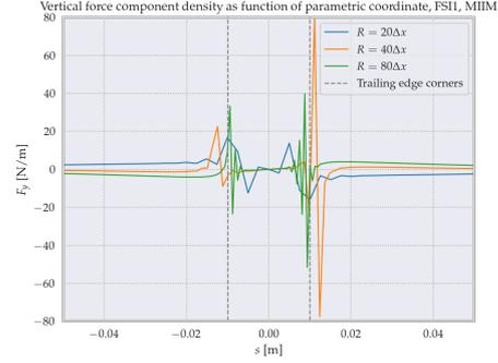
Figure 9.4: Vertical force component density as function of parametric coordinate, for the MIIM for FSII, for three mesh refinement levels.
