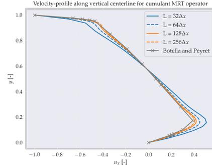
Figure 7.4: Plot of the horizontal velocity component along  $x = L/2$ , at  $t = 200L/u_0$ , for various grid refinement levels, using the cumulant MRT scheme. For the purpose of plotting,  $u_0 = 1.0$  and  $L = 1.0$ .
