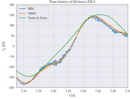
Figure 8.10: Lift as function of time, compared to the reference solution by Turek and Hron [8], using  $R = 20\Delta x$ . Zoomed into the domain  $t \in [7.15, 7.30]$ .
