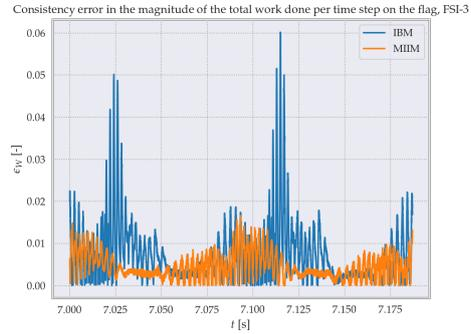
Figure 8.25: Interpolation error in the total work done on the flag per time step, as evaluated from the fluid surface and structure surface, for both the IBM and MIIM.
