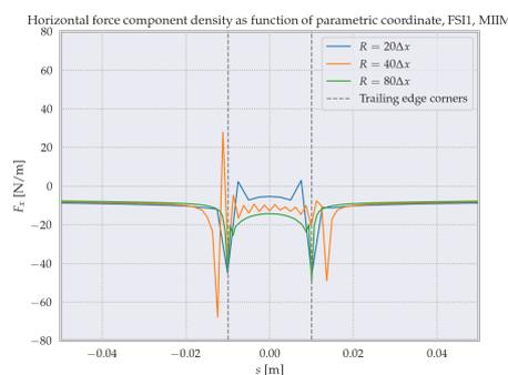
Figure 9.2: Horizontal force component density as function of parametric coordinate, for the MIIM for FSI1, for three mesh refinement levels.
