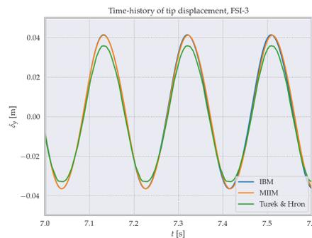
Figure 8.9: Vertical displacement of the tip, compared to the reference solution by Turek and Hron [8], using  $R = 20\Delta x$ .
