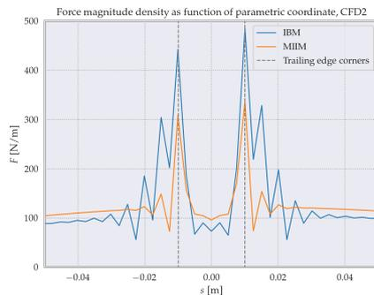
Figure 7.31: Force magnitude density as function of parametric coordinate, for the IBM and MIIM, for CFD2.
