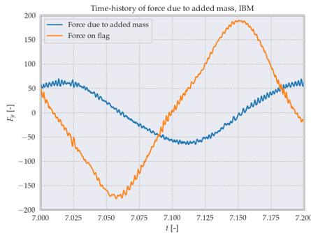
Figure 8.12: Force due to added mass effect over a single period of motion for the IBM, at a grid resolution of  $R = 20\Delta x$ , compared to the total force on the flag.
