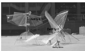
Figure 2.3: The DelFly I, DelFly II and DelFly Micro. The DelFly II is the most established model of the family, according to Tay et al. [20]. Taken from [19, p. 3].
