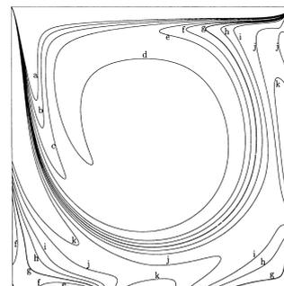
Figure 7.2: Plot of the reference iso-vorticity lines for a lid-driven cavity flow, as per Botella and Peyret. Taken from [92, p. 428].
