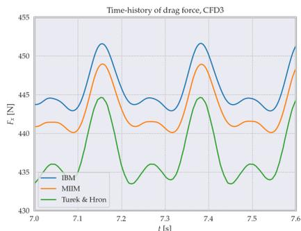
Figure 7.35: Drag as function of time, compared to the reference solution by Turek and Hron [8], using  $R = 40\Delta x$ .
