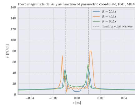
Figure 9.6: Force magnitude density as function of parametric coordinate, for the IBM for MIIM, for three mesh refinement levels.
