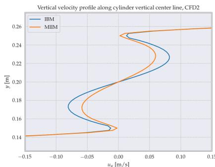
Figure 7.33: Vertical velocity profile along the vertical axis crossing through the center of the cylinder, for CFD2.
