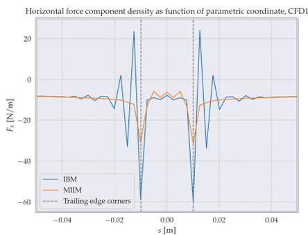
Figure 7.26: Horizontal force component density as function of parametric coordinate, for the IBM and MIIM, for CFD1.
