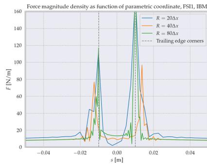
Figure 9.5: Force magnitude density as function of parametric coordinate, for the IBM for FSII, for three mesh refinement levels.
