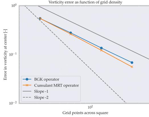
Figure 7.5: Plot of the error in the vorticity at the center of domain ( $x = L/2$ ,  $y = L/2$ ), as function of grid density, for the BGK and cumulant MRT operators.
