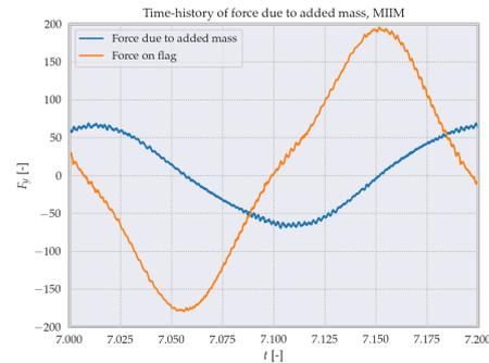
Figure 8.13: Force due to added mass effect over a single period of motion for the MIIM, at a grid resolution of  $R = 20\Delta x$ , compared to the total force on the flag.
