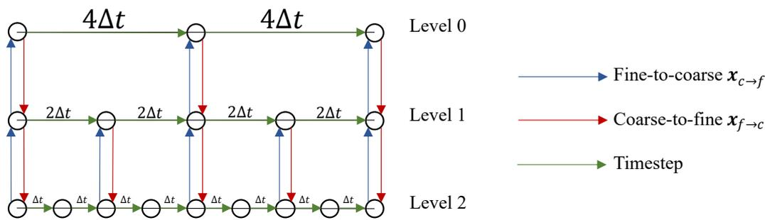
Figure 6.6: Time stepping scheme of the proposed multigrid procedure. The finest grids runs at a time step of  $\Delta t$ ; and every level above runs at a time step twice as long as the previous level. Whenever a parent grid matches up in time with its sub grids, communication between the grids takes place.
