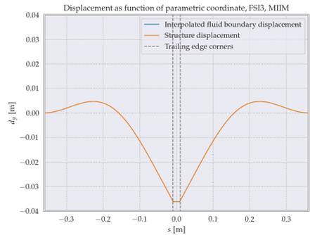
Figure 8.23: Deflection as function of parametric coordinate, for the IBM for FSI3, for both the fluid and structure, the former being interpolated from the latter.
