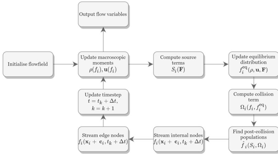
Figure 3.1: Generic sequencing of operations in an LBM simulation.
