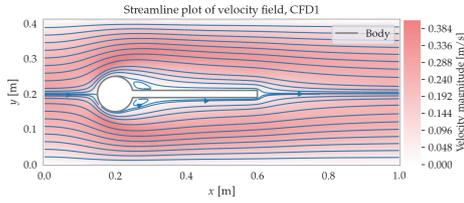
Figure 7.24: Streamline plot of the flow around the cylinder and flag for the MIIM, for CFD1, at a mesh resolution such that  $R = 20\Delta x$ .
