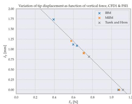
Figure 8.6: Plot of the tip displacement as function of vertical force on the system, for FSI1 and CFD1 benchmark cases.
