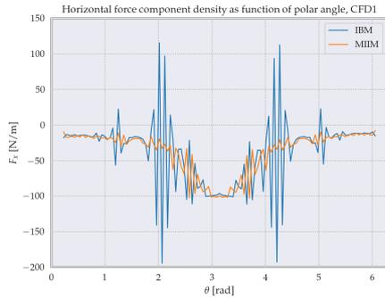
Figure 7.18: Horizontal force component density as function of polar angle, for the IBM and MIIM, for CFD1.
