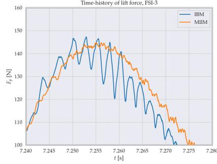
Figure 8.11: Lift as function of time, compared to the reference solution by Turek and Hron [8], using  $R = 20\Delta x$ . Zoomed into the domain  $t \in [7.24, 7.28]$ .
