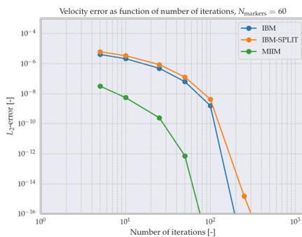
Figure 7.10: Plot of  $L_2$ -error as function of the number of iterations, for a number of markers equal to  $K = 60$ .
