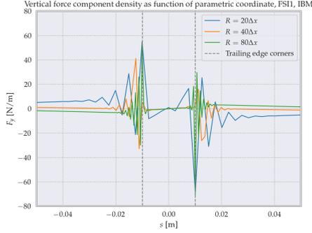
Figure 9.3: Vertical force component density as function of parametric coordinate, for the IBM for FSII, for three mesh refinement levels.
