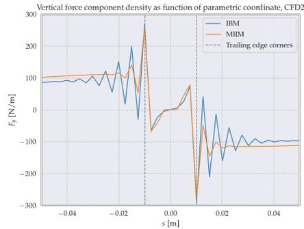
Figure 7.29: Vertical force component density as function of parametric coordinate, for the IBM and MIIM, for CFD2.
