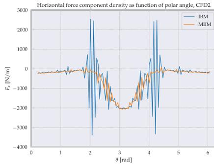
Figure 7.19: Horizontal force component density as function of polar angle, for the IBM and MIIM, for CFD2.
