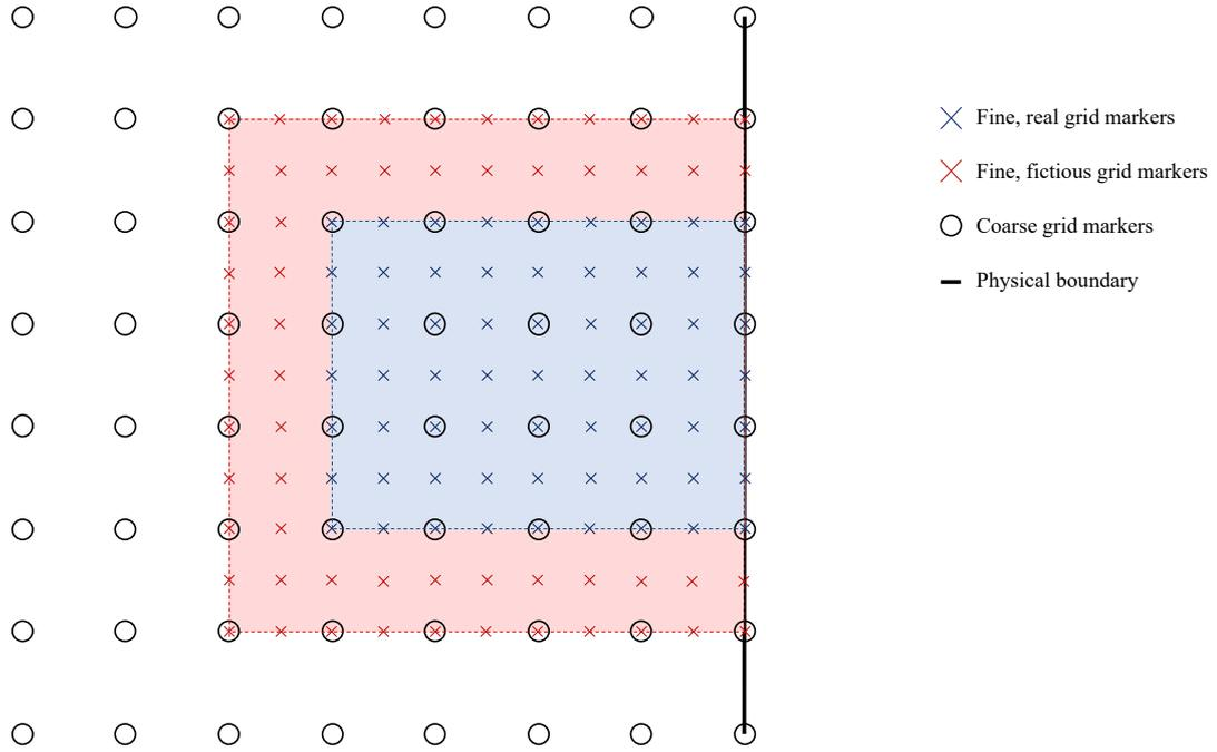
Figure 6.7: Example of a simple multi-grid configuration. In the blue area, information from the fine grid is used to improve the accuracy of the solution at coinciding coarse grid nodes. The red area is an area padded around the blue area, and becomes diluted over time due to lack of physical boundary conditions.
