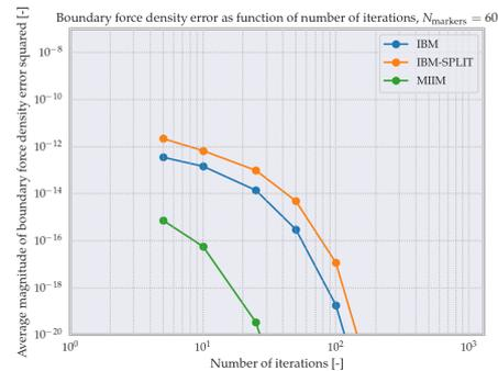
Figure 7.11: Plot of  $\epsilon_F$ -error as function of the number of iterations, for a number of markers equal to  $K = 60$ .
