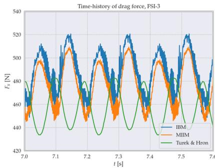
Figure 8.7: Drag as function of time, compared to the reference solution by Turek and Hron [8], using  $R = 20\Delta x$ .
