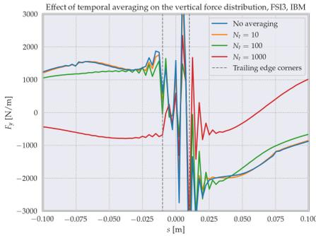
Figure 8.16: Vertical force component density as function of parametric coordinate, for the IBM for FSI3, for three levels of temporal averaging.
