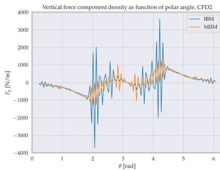
Figure 7.21: Vertical force component density as function of polar angle, for the IBM and MIIM, for CFD2.
