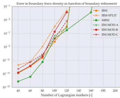
Figure 7.9: Plot of  $\epsilon_F$ -error as function of the number of Lagrangian markers, for  $L = 20\Delta x$ .
