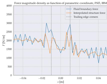
Figure 8.20: Boundary force magnitude density as function of parametric coordinate (zoomed into region around the tip of the flag), for the IBM for FSI3, for both the fluid and structure, the latter being interpolated from the former.
