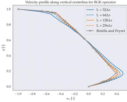
Figure 7.3: Plot of the horizontal velocity component along  $x = L/2$ , at  $t = 200L/u_0$ , for various grid refinement levels, using the BGK operator. For the purpose of plotting,  $u_0 = 1.0$  and  $L = 1.0$ .
