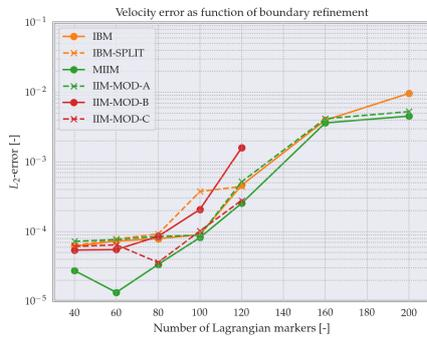
Figure 7.8: Plot of  $L_2$ -error as function of the number of Lagrangian markers, for  $L = 20\Delta x$ .
