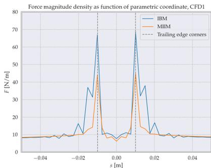
Figure 7.30: Force magnitude density as function of parametric coordinate, for the IBM and MIIM, for CFD1.
