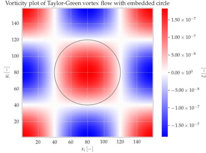
Figure 7.6: Plot of the vorticity at  $t = L/u_0$ , using a grid spacing of  $L = 40\Delta x$ , simulated by the IIM-BASE scheme.
