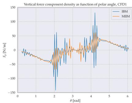
Figure 7.20: Vertical force component density as function of polar angle, for the IBM and MIIM, for CFD1.
