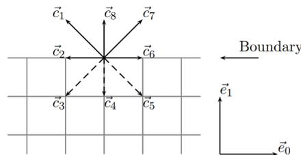
Figure 6.8: Illustration of lattice populations at upper edge of a fluid domain. Taken from [87, p. 54].
