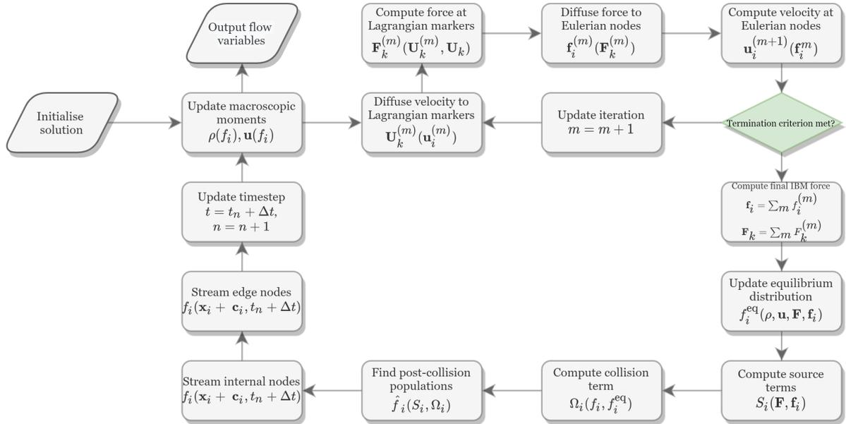
Figure 4.3: Generic sequencing of operations in an IBM-LBM simulation.
