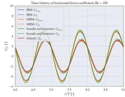
Figure 8.3: Drag as function of time, compared to the reference solution by Suzuki and Inamuro [96], for  $Re = 100$  and  $D = 80\Delta x$ .
