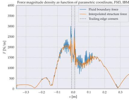
Figure 8.18: Boundary force magnitude density as function of parametric coordinate, for the IBM for FSI3, for both the fluid and structure, the latter being interpolated from the former.
