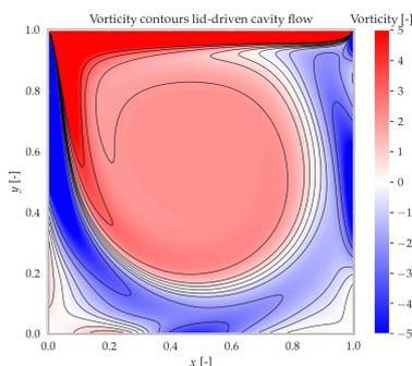
Figure 7.1: Plot of the vorticity at  $t = 200L/u_0$ , using  $N = 257$  nodes in each direction, using the cumulant MRT scheme. For the purpose of plotting,  $u_0 = 1.0$  and  $L = 1.0$ .
