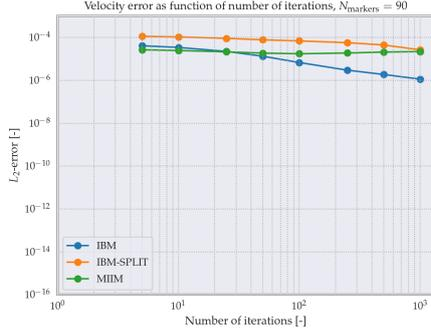
Figure 7.12: Plot of  $L_2$ -error as function of the number of iterations, for a number of markers equal to  $K = 90$ .
