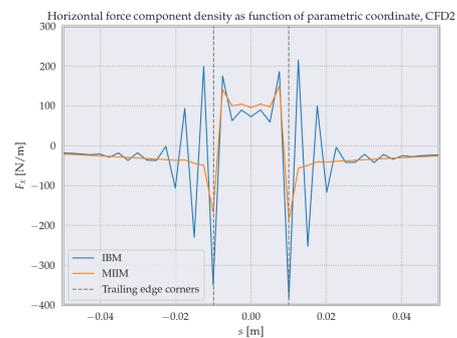
Figure 7.27: Horizontal force component density as function of parametric coordinate, for the IBM and MIIM, for CFD2.
