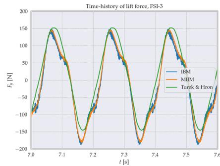
Figure 8.8: Lift as function of time, compared to the reference solution by Turek and Hron [8], using  $R = 20\Delta x$ .
