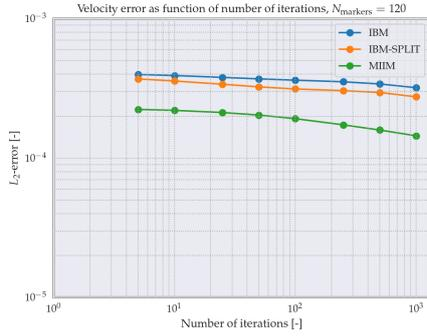
Figure 7.14: Plot of  $L_2$ -error as function of the number of iterations, for a number of markers equal to  $K = 120$ .
