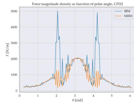
Figure 7.23: Force magnitude density as function of polar angle, for the IBM and MIIM, for CFD2.
