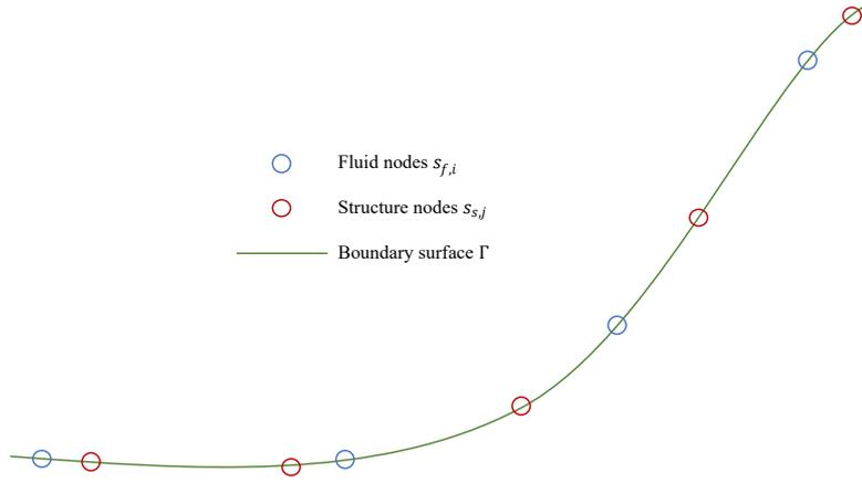
Figure 6.2: Discretisation of a boundary, with fluid nodes (as used by the IBM/MIIM by the fluid solver described in Chapter 4 and 5) and structural nodes (as used by the structural model described in Section 6.1).
