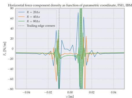
Figure 9.1: Horizontal force component density as function of parametric coordinate, for the IBM for FSI1, for three mesh refinement levels.
