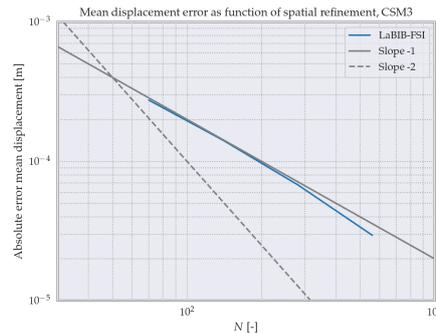
Figure 8.4: Plot of the absolute error of the mean displacement as function of spatial refinement.
