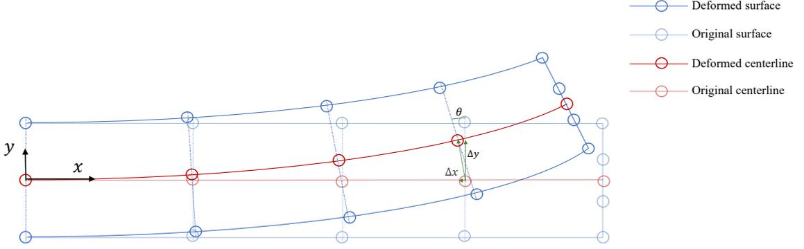
Figure 6.1: Structural model of a cantilevered beam, in its original and deformed position. The displacements at the outer surface nodes can be evaluated directly from the translation and rotation of the beam elements located at the centerline.
