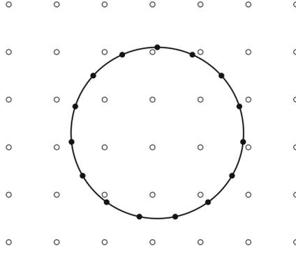
Figure 4.1: Sketch of a cylinder discretised by an Lagrangian mesh, embedded in an Eulerian mesh. Taken from Krüger et al. [2, p. 466].
