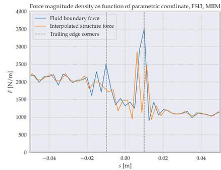
Figure 8.21: Boundary force magnitude density as function of parametric coordinate (zoomed into region around the tip of the flag), for the MIIM for FSI3, for both the fluid and structure, the latter being interpolated from the former.
