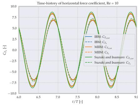
Figure 8.2: Drag as function of time, compared to the reference solution by Suzuki and Inamuro [96], for  $Re = 10$  and  $D = 80\Delta x$ .
