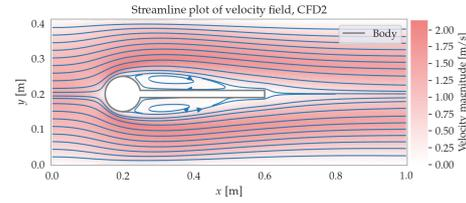
Figure 7.25: Streamline plot of the flow around the cylinder and flag for the MIIM, for CFD2, at a mesh resolution such that  $R = 20\Delta x$ .
