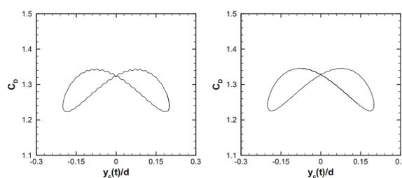
Figure 2.7: Variation over time of the drag coefficient of an oscillating cylinder, at  $Re = 185$ , using a 'bare' interpolating function (left) and its smoothed variant (right). Taken from [39, p. 7833].
