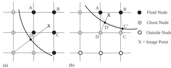
Figure 2.5: Interpolation stencils for two types of boundary intersections. In (a), the image point is reflected into a square cell. In (b), the image point is reflected into a cell that is cut by the boundary. Taken from [33, p. 487].
