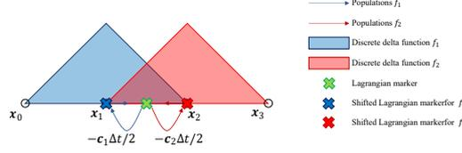
Figure 5.3: Interpolation zone for a Lagrangian marker in the MIIM in a one-dimensional stencil.
