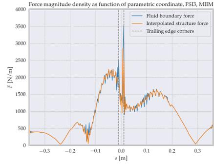
Figure 8.19: Boundary force magnitude density as function of parametric coordinate, for the MIIM for FSI3, for both the fluid and structure, the latter being interpolated from the former.
