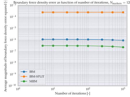
Figure 7.15: Plot of  $\epsilon_F$ -error as function of the number of iterations, for a number of markers equal to  $K = 120$ .
