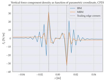
Figure 7.28: Vertical force component density as function of parametric coordinate, for the IBM and MIIM, for CFD1.
