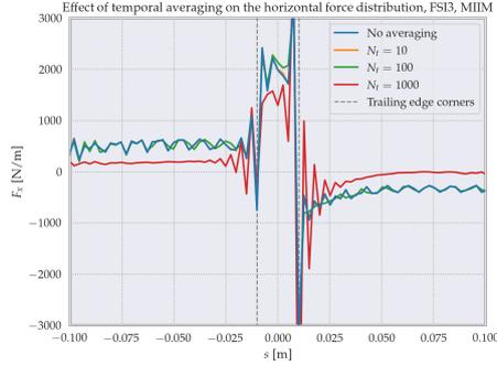
Figure 8.15: Horizontal force component density as function of parametric coordinate, for the MIIM for FSI3, for three levels of temporal averaging.
