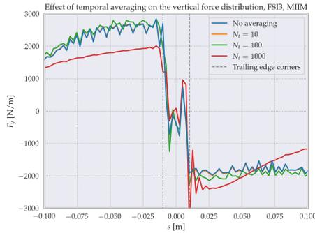
Figure 8.17: Vertical force component density as function of parametric coordinate, for the MIIM for FSI3, for three levels of temporal averaging.
