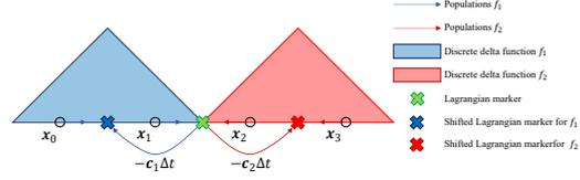
Figure 5.2: Interpolation zone for a Lagrangian marker in the IIM in a one-dimensional stencil.
