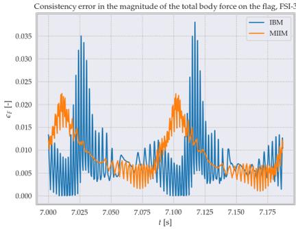
Figure 8.24: Interpolation error in the total boundary force acting on the flag, as evaluated from the fluid surface and structure surface, for both the IBM and MIIM.
