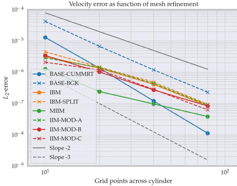
Figure 7.7: Plot of  $L_2$ -error as function of number of grid refinement for a constant Lagrangian marker density.
