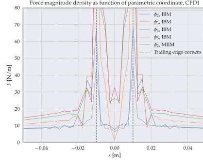
Figure 9.8: Plot of the boundary force distribution at the tip of the flag, for different Mach numbers, for CFD1 at a mesh discretisation such that  $R = 20\Delta x$ .
