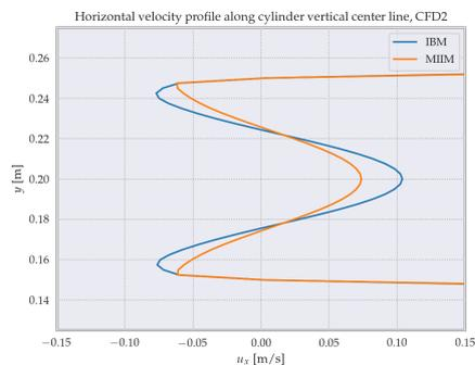
Figure 7.32: Horizontal velocity profile along the vertical axis crossing through the center of the cylinder, for CFD2.
