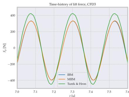
Figure 7.36: Lift as function of time, compared to the reference solution by Turek and Hron [8], using  $R = 40\Delta x$ .
