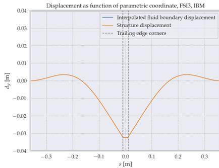
Figure 8.22: Deflection as function of parametric coordinate, for the IBM for FSI3, for both the fluid and structure, the former being interpolated from the latter.
