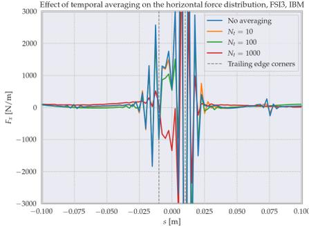
Figure 8.14: Horizontal force component density as function of parametric coordinate, for the IBM for FSI3, for three levels of temporal averaging.
