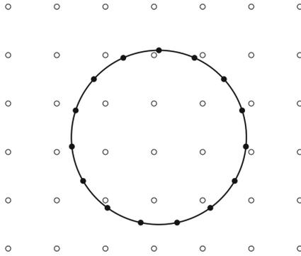
Figure 2.4: Sketch of a cylinder discretised by an Lagrangian mesh, embedded in an Eulerian mesh. Taken from Krüger et al. [2, p. 466].
