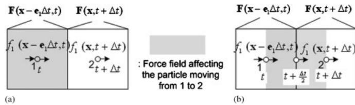
Figure 4.4: Difference between default-forcing (a) and split-forcing (b) with regards to how the force acting on a population at  $\mathbf{x}_n$ , travelling in the direction  $\mathbf{c}_i$ , is computed. Taken from [35, p. 1138].
