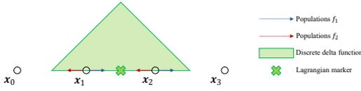
Figure 5.1: Interpolation zone for a Lagrangian marker in the IBM in a one-dimensional stencil.
