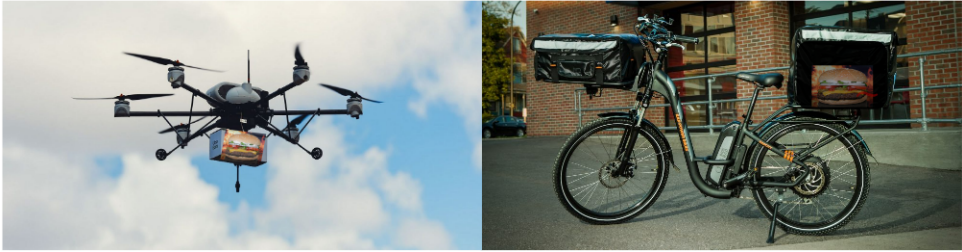
Figure 2.3: Example of a fast-food delivery quad-copter drone, adapted from ([111]); and a typical fast-food delivery E-bike with an integrated delivery cargo box, adapted from ([191]).
