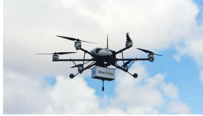
Figure 1.2: Modified DJI matrice 600 copter transporting fast food meals for Uber Eats, adopted from [111].
