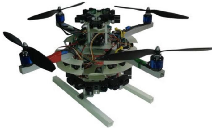
**Figure 4-5:** The AQopter18 equipped with 12 ultrasonic sensors and 16 ( $2 \times 8$ ) infrared sensors [19].
