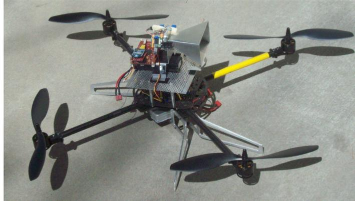
**Figure 4-3:** Quadrotor Equipped with RADAR Sensor [41].
