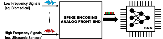
Fig. 1: Illustration of sensory signal processing pipeline using a general purpose analog front end and SNN.
