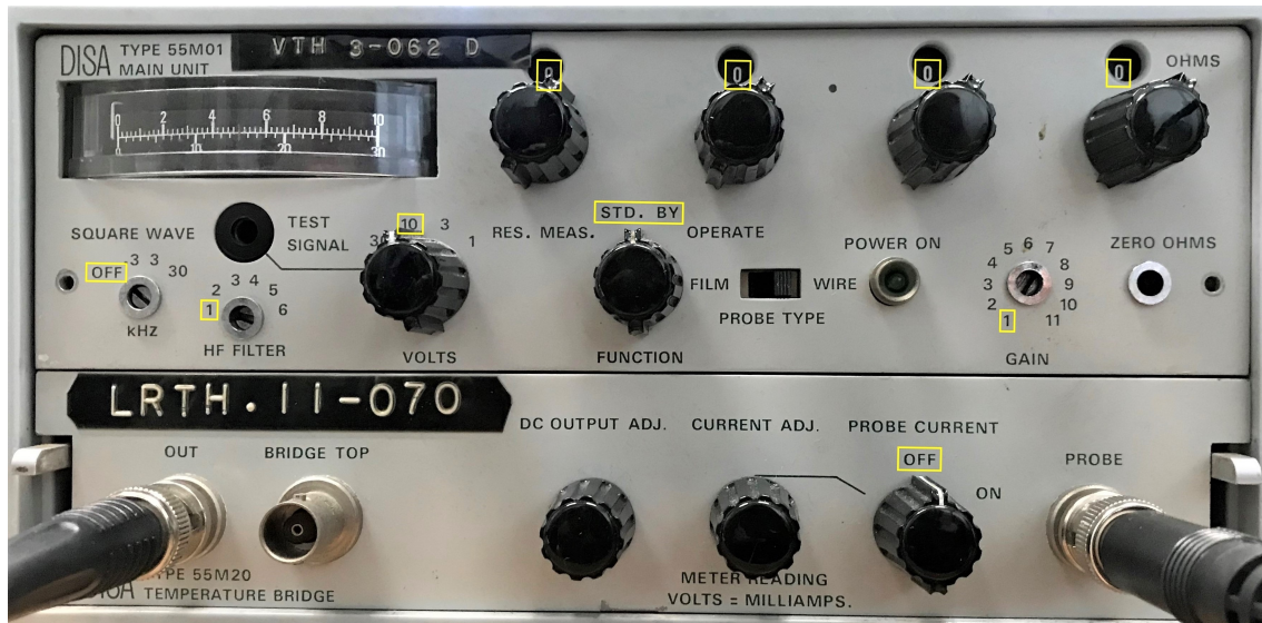
Figure C.2: Initial settings for the DISA 55M constant-current anemometer
