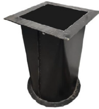
Figure 4.1: Nozzle extension "Delft 50×50" [72]
