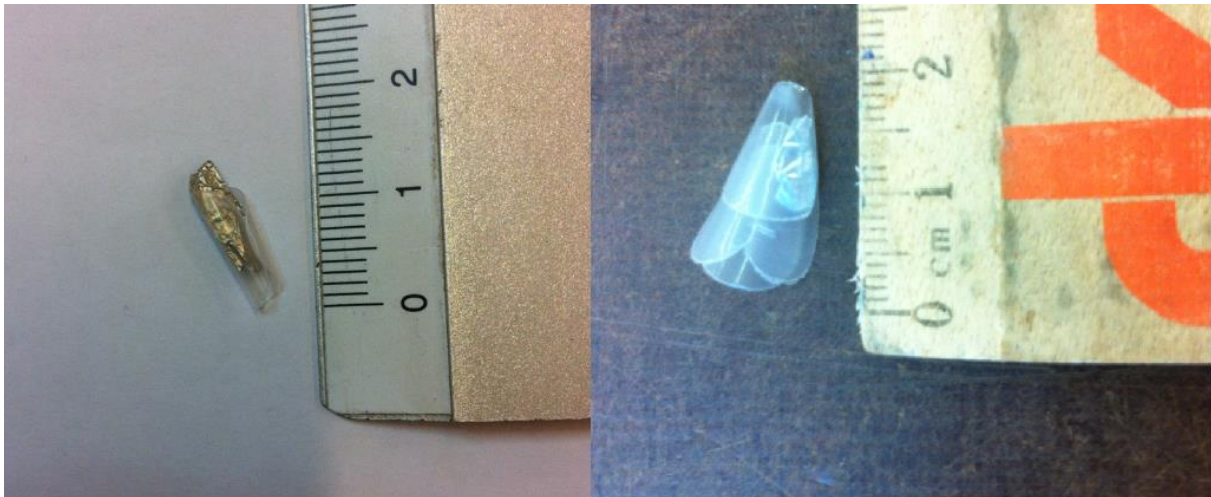
Figure 3.2 Aluminium particle wrapped in LDPE particles.
