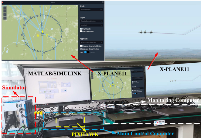
Fig. 1. Experiment prototype of the Links-RT UAV platform.
