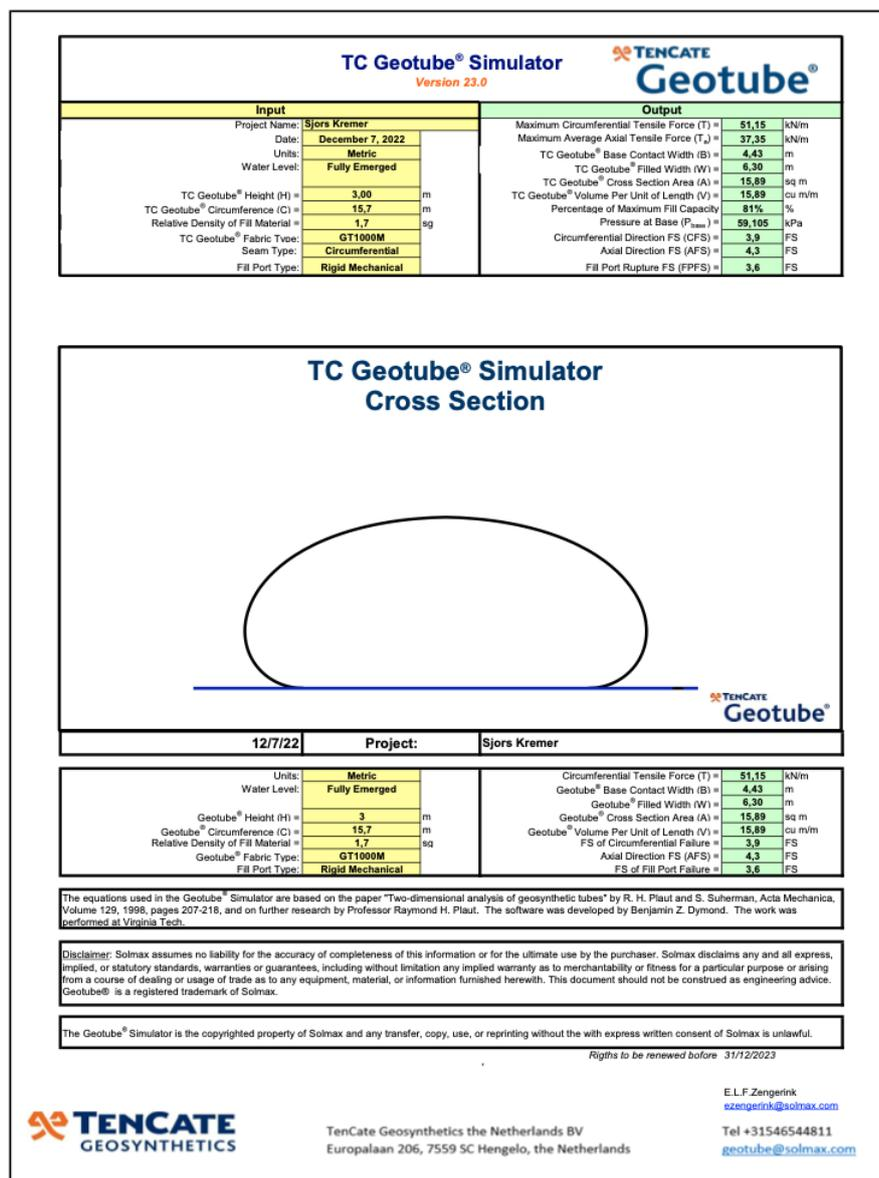
Figure B.1: GeoTube Simulator emerged
