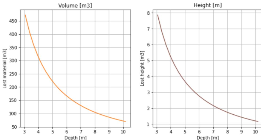
Figure 3.8: Lost volume and core height after a six hour storm
