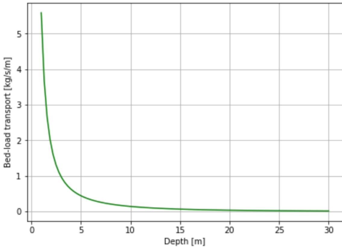
Figure C.1: Bed-Load transport over depth in storm conditions [ $kg/s/m$ ]
