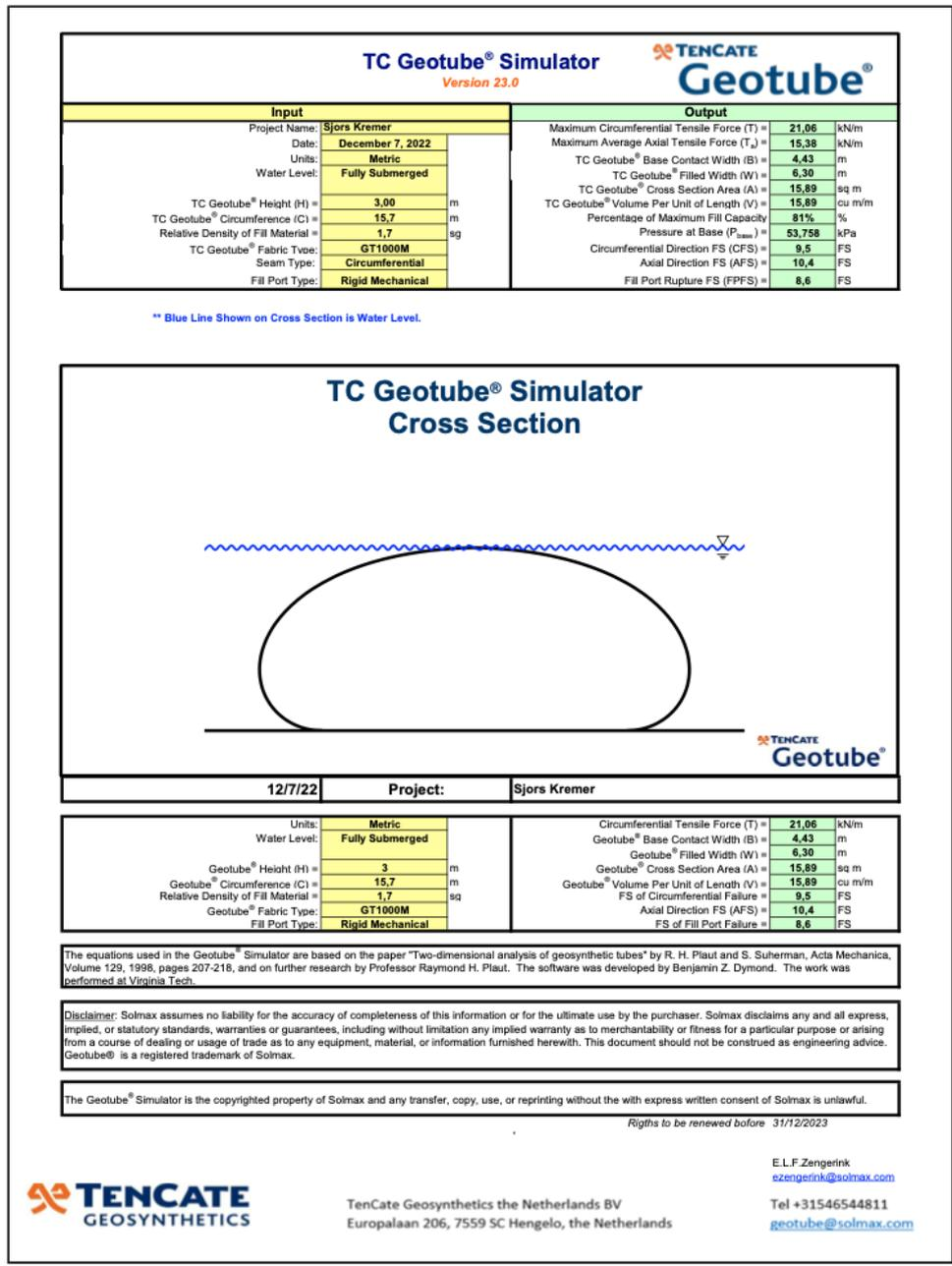
Figure B.2: GeoTube Simulator submerged
