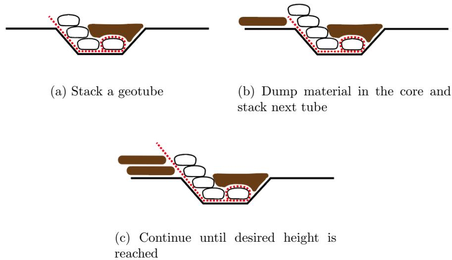
Figure 3.4: Stacking process geotubes
