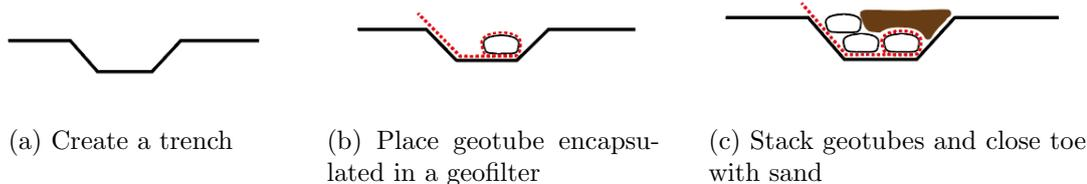
Figure 3.2: Construction self healing toe
