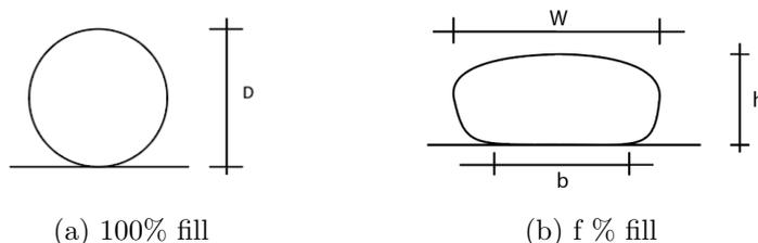
Figure 3.1: Dimensions geotube
