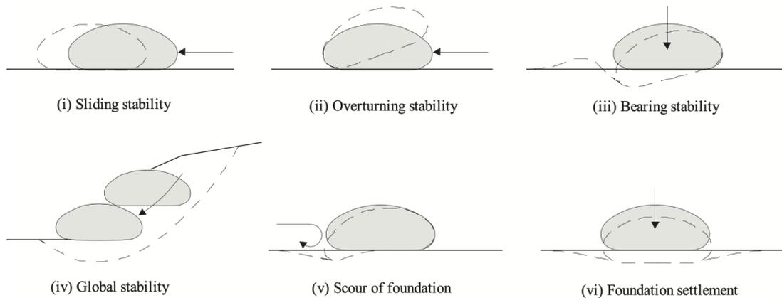
Figure 2.3: External failure mechanisms (Lawson 2006)
