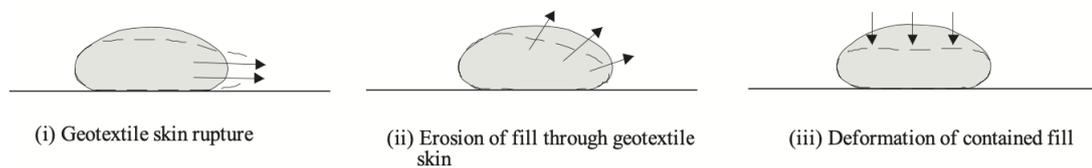
Figure 2.4: Internal failure mechanisms (Lawson 2006)
