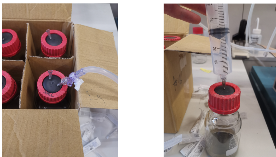
Figure 4.2: Flushing the anaerobic samples and pressurising the aerobic samples [Author's photos]
