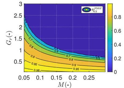
Figure 1: efficiency of a Fly-Gen AWES with the optimal circular flight path ( $\eta_{Cl}^{max}$ ) for each condition expressed by  $M$  and  $G_r$ . The blue region represents the conditions for which the kite cannot fly.
