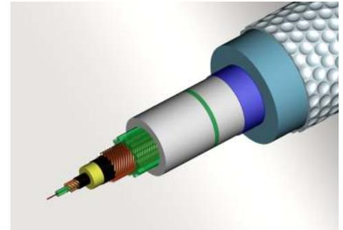
*Scalable, fatigue life optimized, windable, multimegawatt electromechanical tether design for fly-gen AWE systems*
