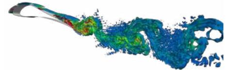
*DDES simulation of an optimised airfoil-slat combination.*
