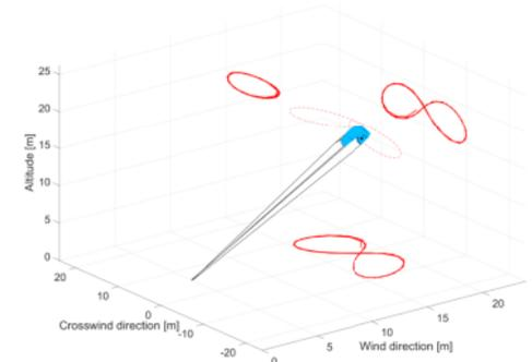
*Kite flight of a figure-eight trajectory using a nonlinear guidance law with a proportional controller [5].*
