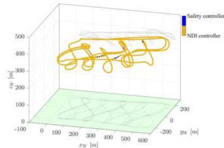
*Multiple pumping cycles using the hybrid control law. A controller using Nonlinear Dynamic Inversion (NDI) [2] is used as a baseline controller and the safety controller is only engaged when a tether rupture is predicted to occur. While the safety controller is only activated rarely, its effect is quite significant.*
