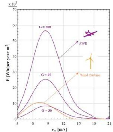
Considering that the average wind speed is 2.78 m/s, we computed the maximum specific AEP of an AWE to be 0.362, 1.087, and 2.415 MWh for effective glide ratios of 30, 90, and 200. For a conventional wind turbine, we computed 0.493 MWh. Given the capacity factor of both technologies, this resource could be available at least 40% [2].
