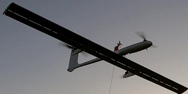
*TwingTec pilot aircraft captured by the wing tip camera.*
