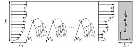
Side view of the computational domain used for co-simulation of turbulent boundary layers and AWE parks. The dimensions in streamwise, spanwise and vertical directions are  $L_x = 10$  km,  $L_y = 4$  km, and  $L_z = 1$  km, respectively. The downstream position of the first row of AWE systems is  $L_1 = 1$  km [3].
