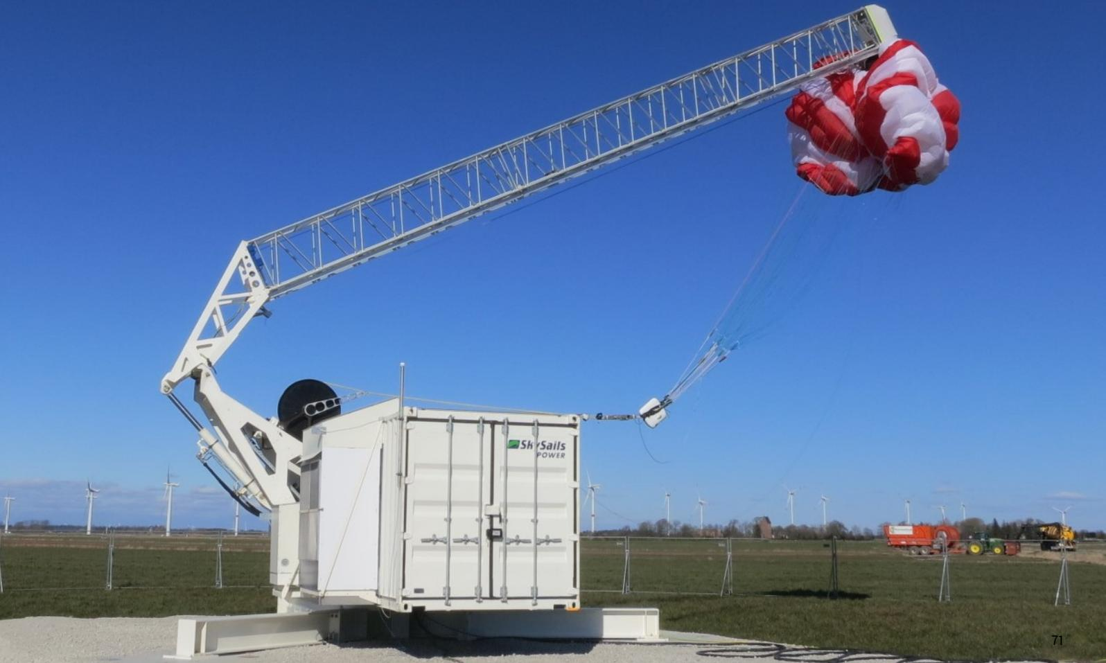
*SkySails Power PN-14 system with inflated kite connected to mast.*
