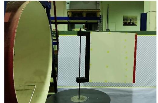
*Wind-tunnel test to identify the flow resistance of various tether markers including mount.*
