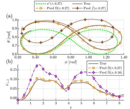
Predicted trajectories with parameter  $v_{\theta\phi}/r$ . Orange: proposed method, brown: black-box nonlinear identification, purple: without  $v_{\theta\phi}/r$  modeling.
