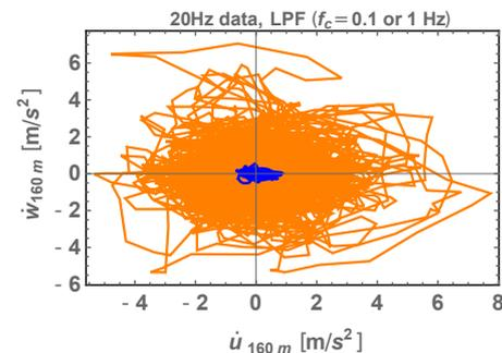
10-minute streamwise/vertical acceleration space: Høvsøre offshore sector, 160m height, sampled at 20Hz. Filtered (O2 Butterworth) for characteristic response times of 10s (blue) and 1s (orange).
