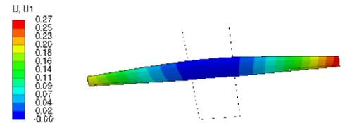
Wing deflection in m (scaled by factor 5) in direction perpendicular to flight for 80 m/s, a vertical circular path with radius 265.5 m and 0° AOA.
