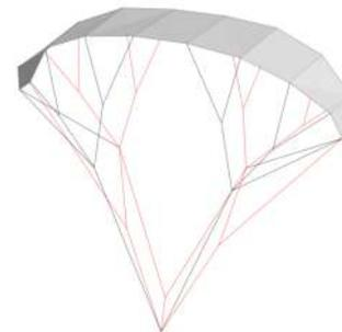
*The PSM for a fully powered kite. Red lines are bridles attached to the trailing edge and black to the leading edge.*
