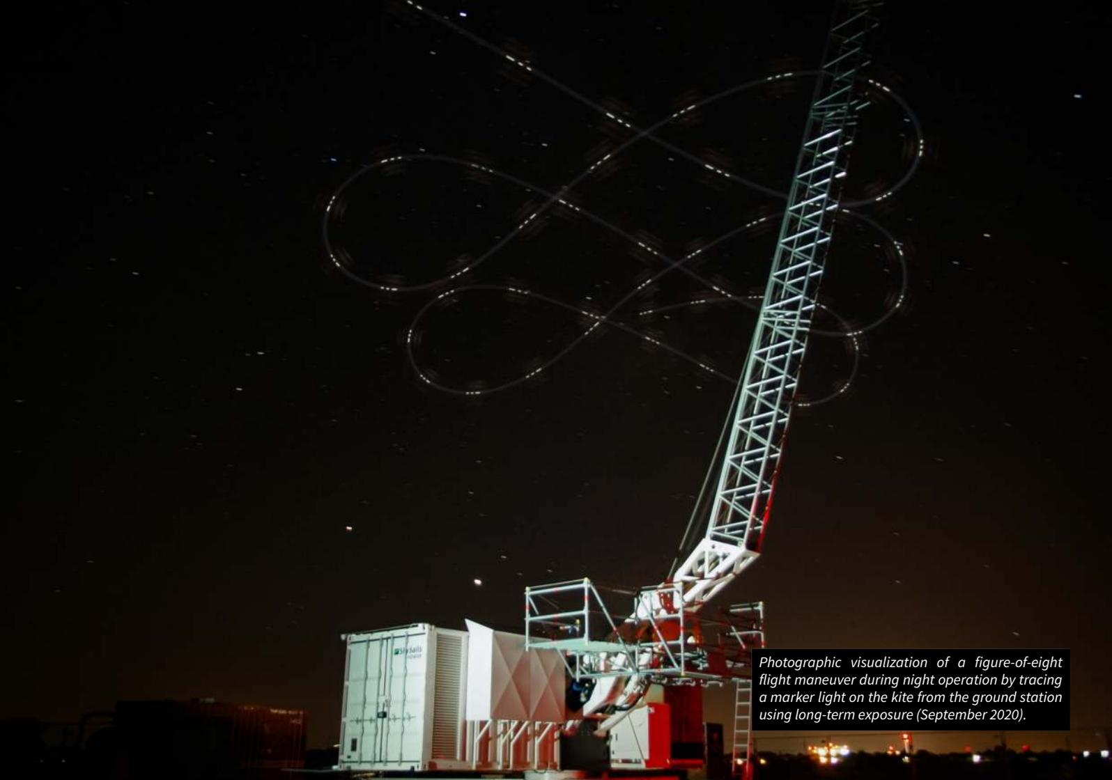
*Photographic visualization of a figure-of-eight flight maneuver during night operation by tracing a marker light on the kite from the ground station using long-term exposure (September 2020).*
