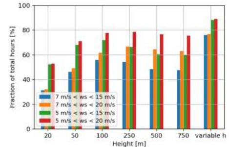
*Fraction of time where conditions are suitable for AWES operation at several heights at the AWES test site Farsund Airport (Norway). There is an upper and lower limit to the windspeed "ws" shown by the different colors. "variable h" includes the ability of the system to adjust its height of operation to the optimal meteorological conditions.*
