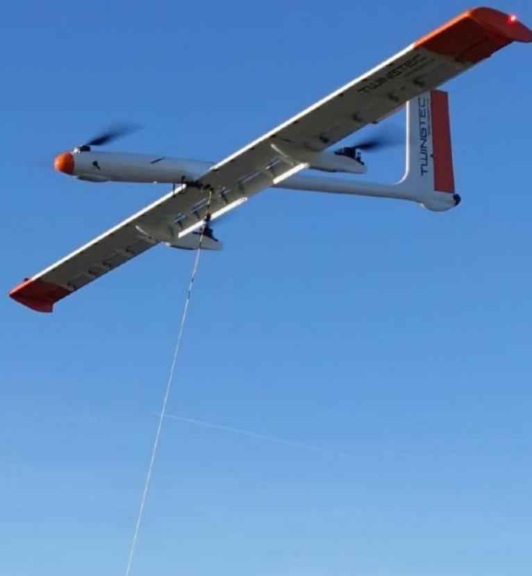
*TwingTec pilot system lifting off from its launch platform.*
