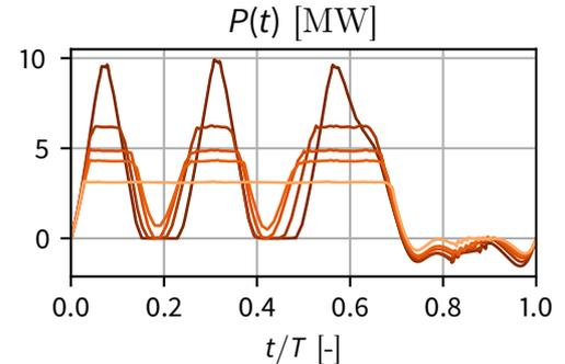
*Possible mechanical power output profiles of a utility-scale pumping single-aircraft system on the Pareto efficiency front of average power vs. PAPR.*
