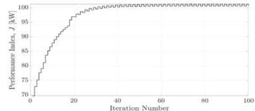
*Example performance improvement resulting from the use of ILC for figure-8 flight path adaptation.*
