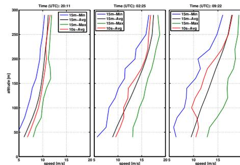
*Lidar measurements of vertical wind shear conditions during daylong operation of the SkySails 60kN power prototype. Notable are significant changes in average wind speed and wind shear situation over time. During night (at 20:11 and 2:25) temporal variation (range min - max) is decreasing with altitude.*
