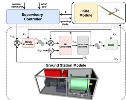
Control architecture integrating the supervisor controller with the GSM and KM, detailing the GSM cascade controller. .
