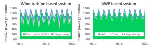
Comparison of the contribution to total power demand from wind, other and energy storage. Due to the more sustained power generation at lower wind speeds airborne wind energy requires much less contribution from other power generation sources.
