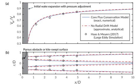
Comparison of our entrainment wake models with the simulation of Haas & Meyers [1] for the laminar inflow case. Similar agreement is found for turbulent inflow [2]. (a) Wake velocity. (b) Wake cross section.
