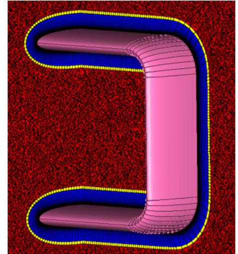
Example of box-wing meshing with cut planes in  $x$  and  $y$ .
