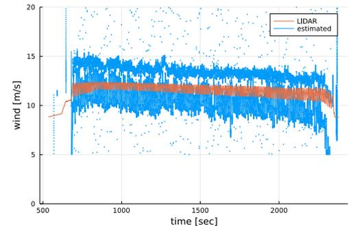
*Experimentally gathered wind speed during a normal production flight with only navigation sensor as input, compared to LIDAR measurements in red.*
