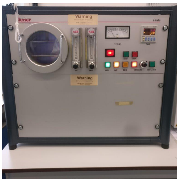
Figure 3.6: Optical photograph of the front control panel of the Diener Femto plasma setup used for surface treatment
