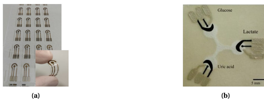
Figure 2.13: Examples of inkjet printed electrodes with (a) the resulting electrode of Figure 2.12 [65] and (b) shows a paper based electrochemical sensor for 3 different analytes [63].
