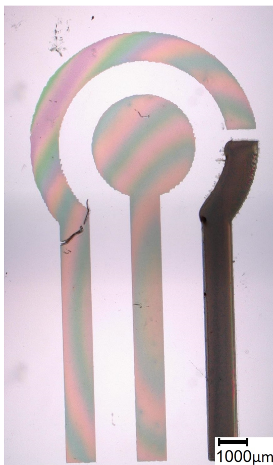
Figure 4.31: Optical microscopy image of a diamond three-electrode sample after CVD diamond growth. Print seeding with diamond NPs was done on an air-exposed, oxygen-plasma treated silicon substrate. The reference electrode (lower right structure) was print-coated with silver ink.
