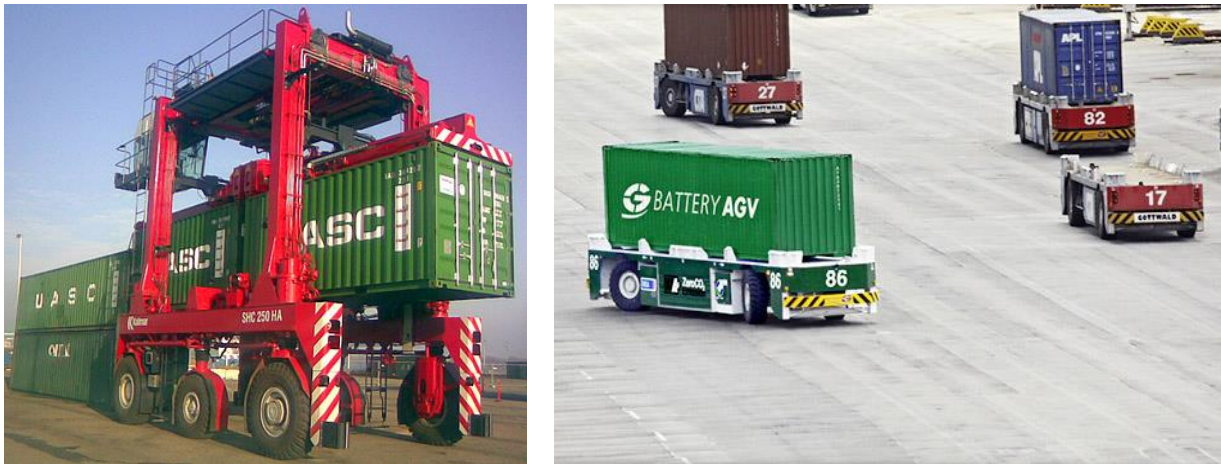
Figure 8 – On the left side an ALV in a container terminal (SAE, 2008) and on the right side an AGV in a container terminal (Demag, n.d.)
