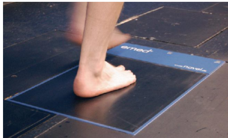
Figure 19. A platform-based foot plantar pressure sensor emed® by Novel (Abdul Razak et al., 2012)
