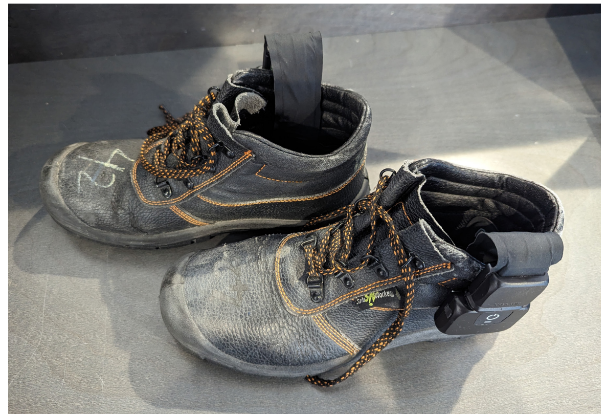
Figure 35. Safety shoes with pressure measurement insoles
