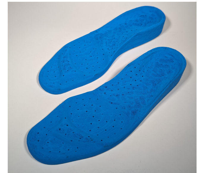
Material: Varioshore 3D Printed inlay sole without fabric
