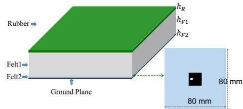
Fig. 1. Proposed antenna design. The thickness of the rubber is  $h_R = 3$  mm. The material inside of the cavity is felt with a permittivity close to 1 and a height of  $h_{F1} = 15$  mm and the patch antenna is located on top of a felt layer with an approximate thickness of  $h_{F2} = 1.5$  mm.
