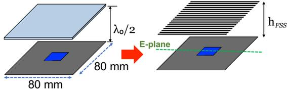
Fig. 6. Equivalence between dielectric superlayer and inductive FSS.
