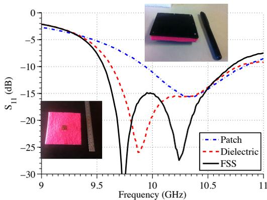
Fig. 11. Comparison of the experimental  $S_{11}$ .
