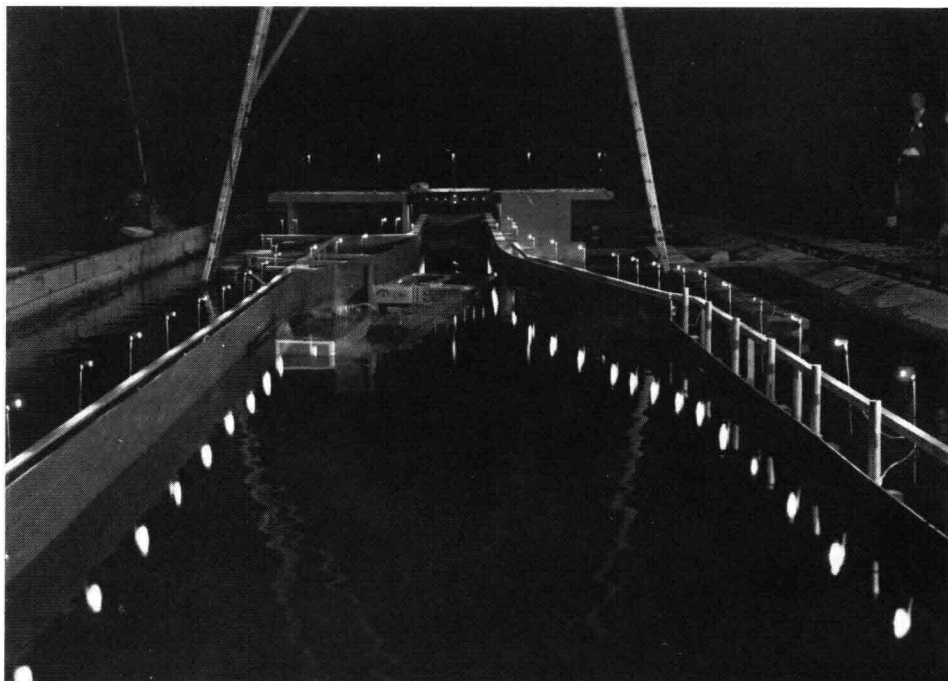
Photograph 5. Optical guidance by using a guiding light system in the Volkerak Lock model (1:25 m)
