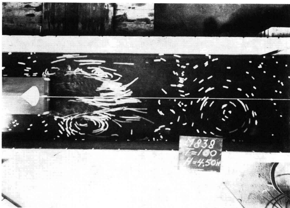
Photograph 11. Flow pattern caused by the propellers of a push tow leaving the lock (model)
