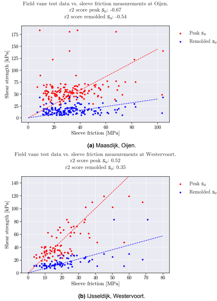
Figure 4.14: Field vane test results vs the measured sleeve friction at the two test sites.
