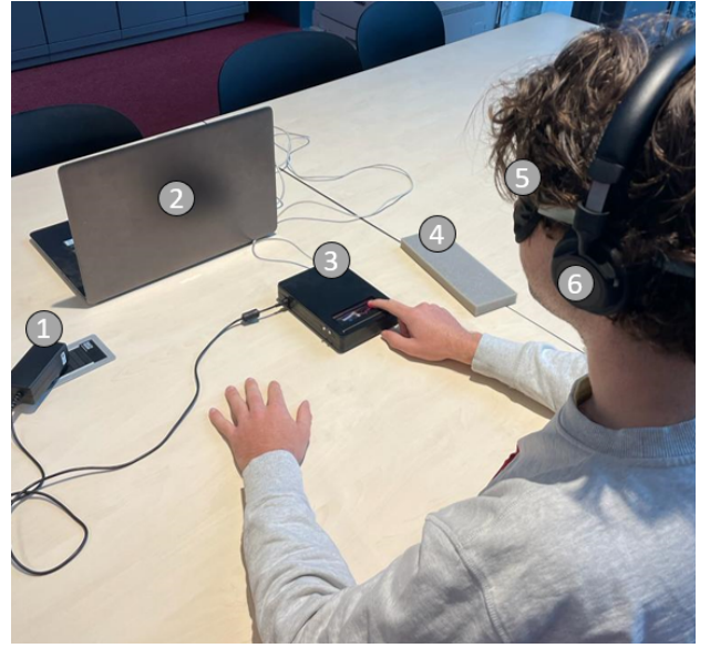
Fig. 5: Experimental setup, with (1) Power supply, (2) Laptop, (3) Haptic Device, (4) Armrest, (5) Blindfold, (6) Noise cancelling headphones
